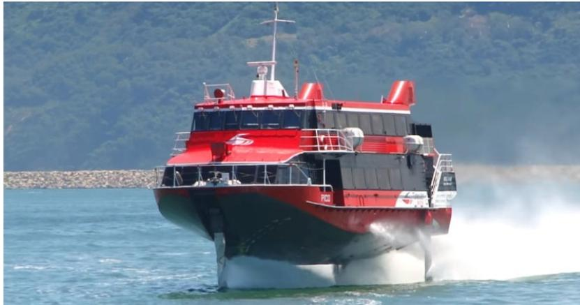
Figure 1.4: *The Boeing 929 Jetfoil Waterjet-Propelled Hydrofoil*
