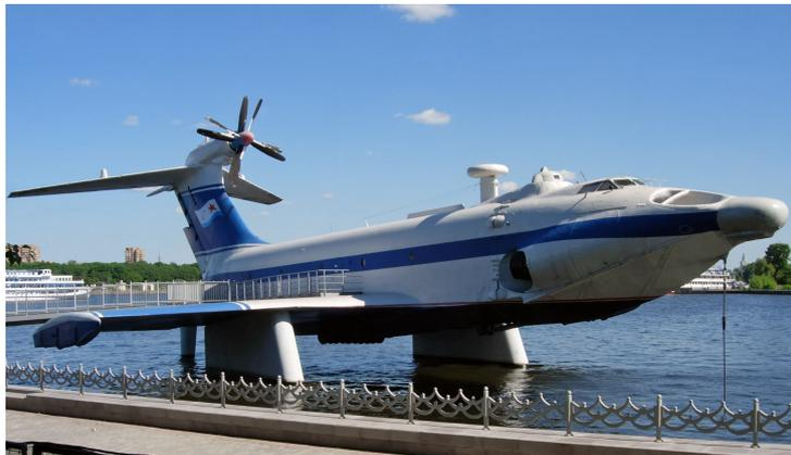
Figure 1.6: *The Alekseev A-90 Orlyonok ekranoplan*
