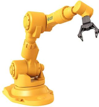
Figure 1.1. Example of base-fixed robot
