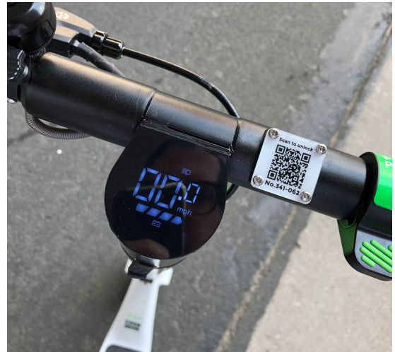
Figure 1.2: E-scooter handlebar with dashboard, QR code and power lever [7].
