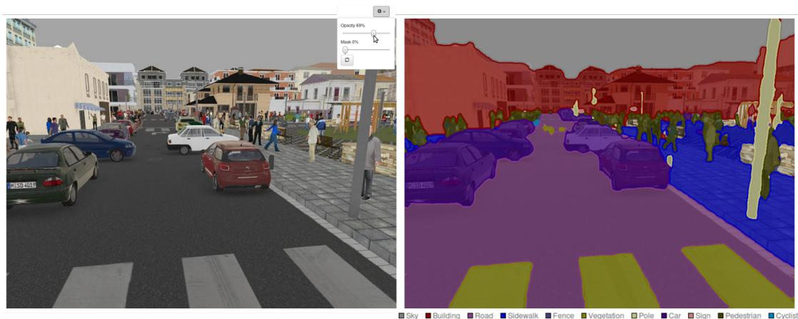
Figure 4.9. Un esempio di Semantic Segmentation applicata in ambito automotive. Credit to <https://bit.ly/3rSfFDI>
