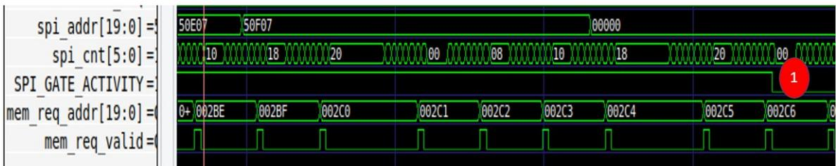
Figure 4.7: Synfire chain with 8 neurons: configuration phase ends as soon as SPI\_GATE\_ACTIVITY is lowered. This lets ODIN run the synfire chain.
