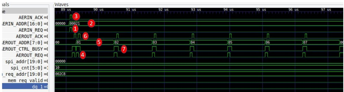
Figure 4.8: Synfire chain with 8 neurons: neuron 0 is stimulated by a virtual synapse event (points 1-3), then every neuron of the synfire chain fires in sequence (points 4-7).
