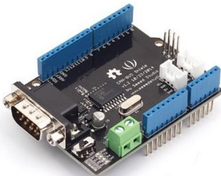
Fig. V.1: CAN-BUS Shield V2.0 [24]
