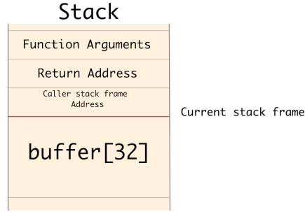
Figure 2.3. Stack before payload injection
