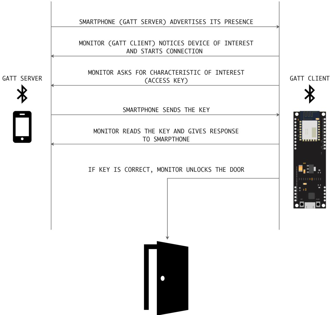
Figure 4.2. Here the architecture of the monitoring system, as well as the exchange of data between the two main parts, is schematized
