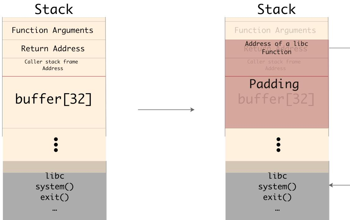
Figure 2.2. Exploitation of a buffer overflow for a return-to-libc attack
