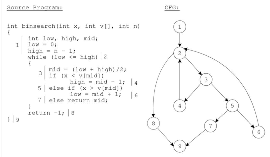
Figure 2.6. Example of Control Flow Graph
