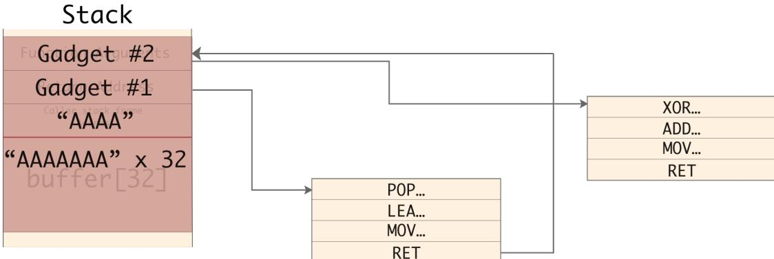
Figure 2.5. Stack's situation after ROP
