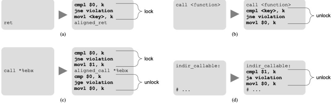
Figure 2.8. Code Instrumentation proposed in [3] in the different typologies of control transfer sites.
