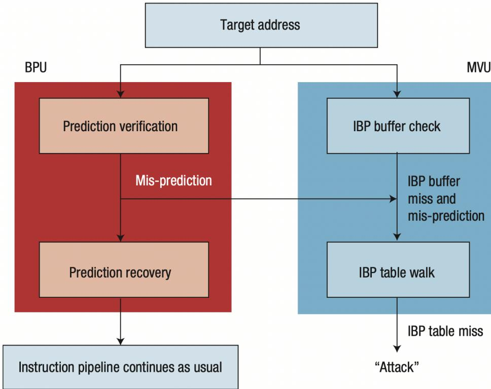
Figure 2.14. Mis-prediction Validation Unit. Image taken from [20]
