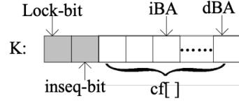
Figure 2.10. Layout of K in coarse grain CFLC
