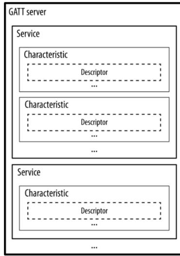
Figure 4.3. GATT server schematic, picture taken from [6]
