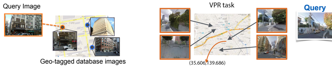
Figure 1.1. On the left the distinction between the gallery and the query; on the right an example of a VPR task.
