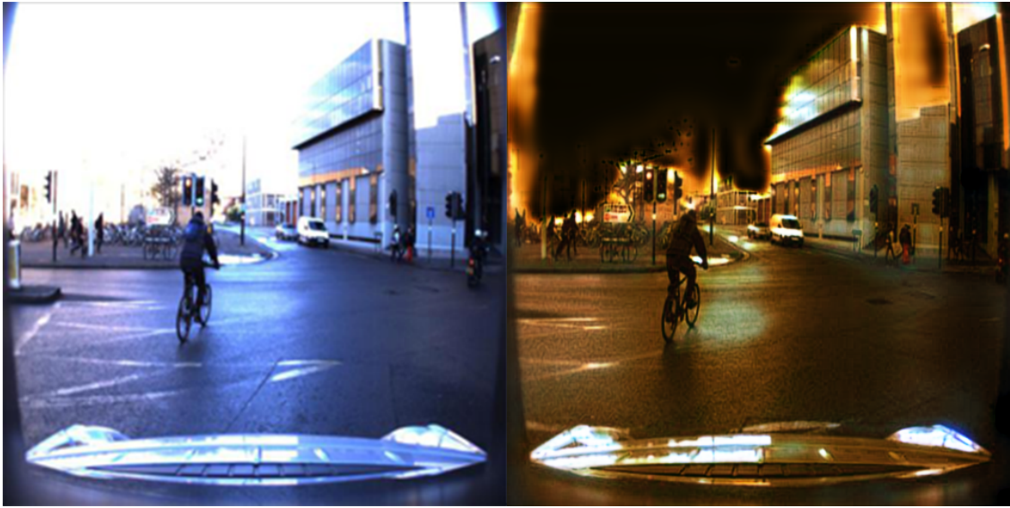
Figure 4.8. On the left a picture from Oxford RobotCar taken at daytime. On the right the same picture shifted to night domain thanks to FastCUT.
