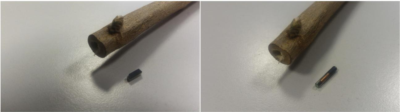
Figure 2.21: Tag Integration Into Branch (UHF Left, LF Right)
