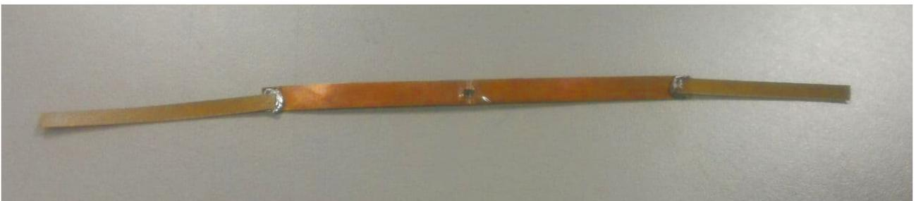
Figure 2.19: UHF Tag Applied on the Custom Antenna
