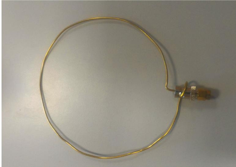
Figure 2.16: Loop Antenna Implementation
