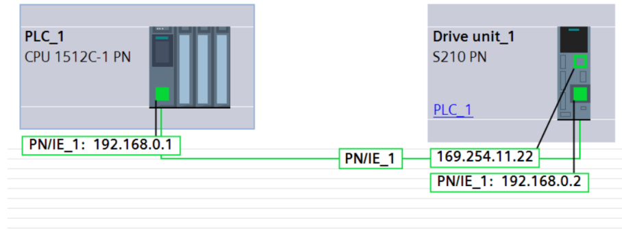
Figure 45: Link between drive and PLC
