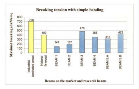
Breaking tensions obteined in laboratory tests reached great results, particularly for beams realised with melamminic glue which reached a breaking as good as heart-wood's one. The beam made disposing laminae vertically even exceeded natural firwood's breaking tension. All beams have regular deformations (arrows and lenghtenings/shortenings of the centre-line section) both when adding load and when taking it away.
