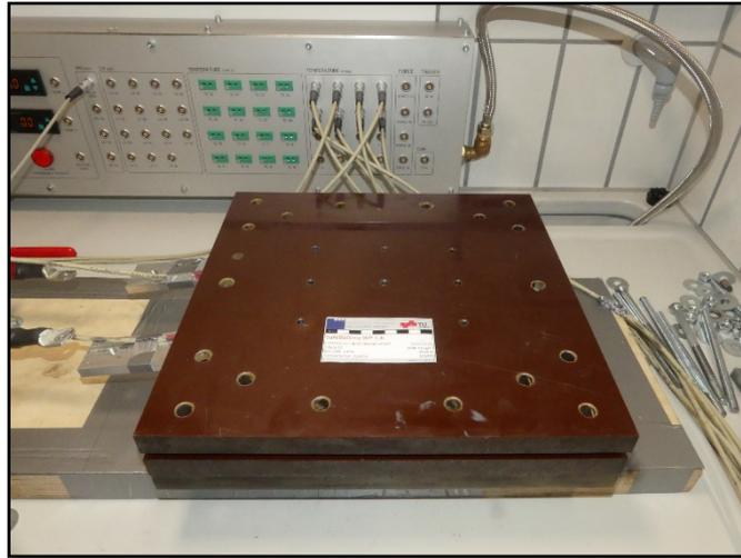
*Figure 61 - Addition of superior Pertinax plate*
