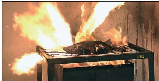
*Figure 21 - Explosion of battery due to abusive test (via Web)*
