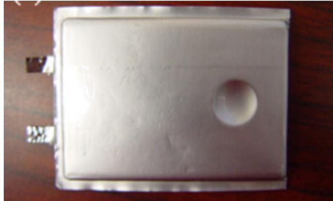
*Figure 24 – Example of denting on a pouch battery*
