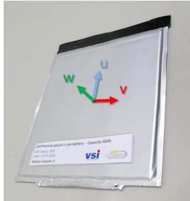
Figure 31 - Example of battery under test
