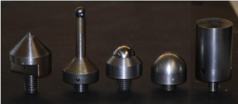
*Figure 37 - Five punch heads used in indentation tests<sup>18</sup>*
