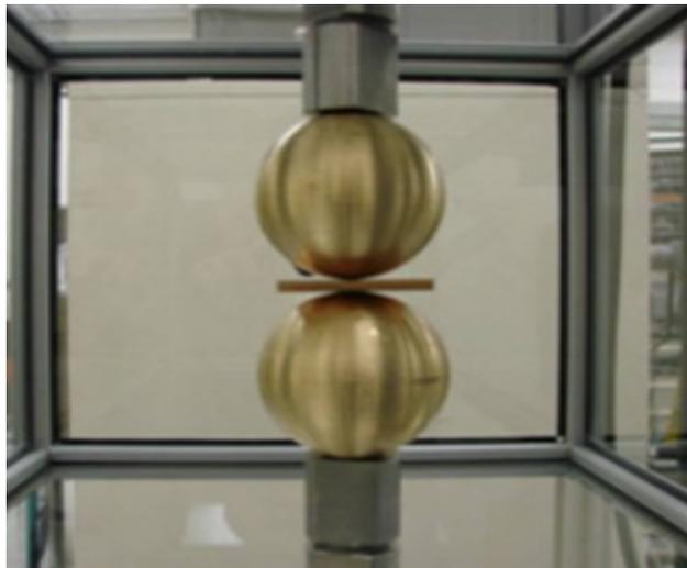
*Figure 26 – Example of pinch test*
