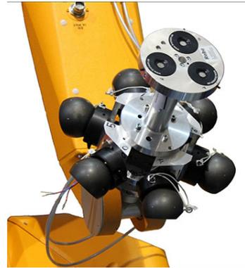
Figure 1.6: Robot with 6 reflector attached to its end-effector [4]
