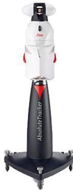
Figure 1.5: Leica laser tracker
