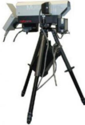
Figure 1.6: Traffic monitoring system
