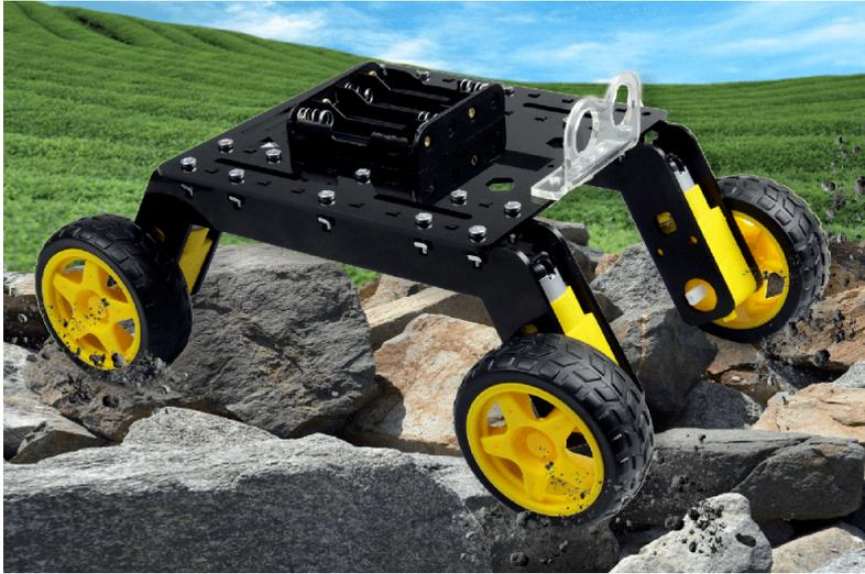
Figure 6.1: 4WD Four wheel steering robot with suspensions for autonomous navigation and outdoor applications
