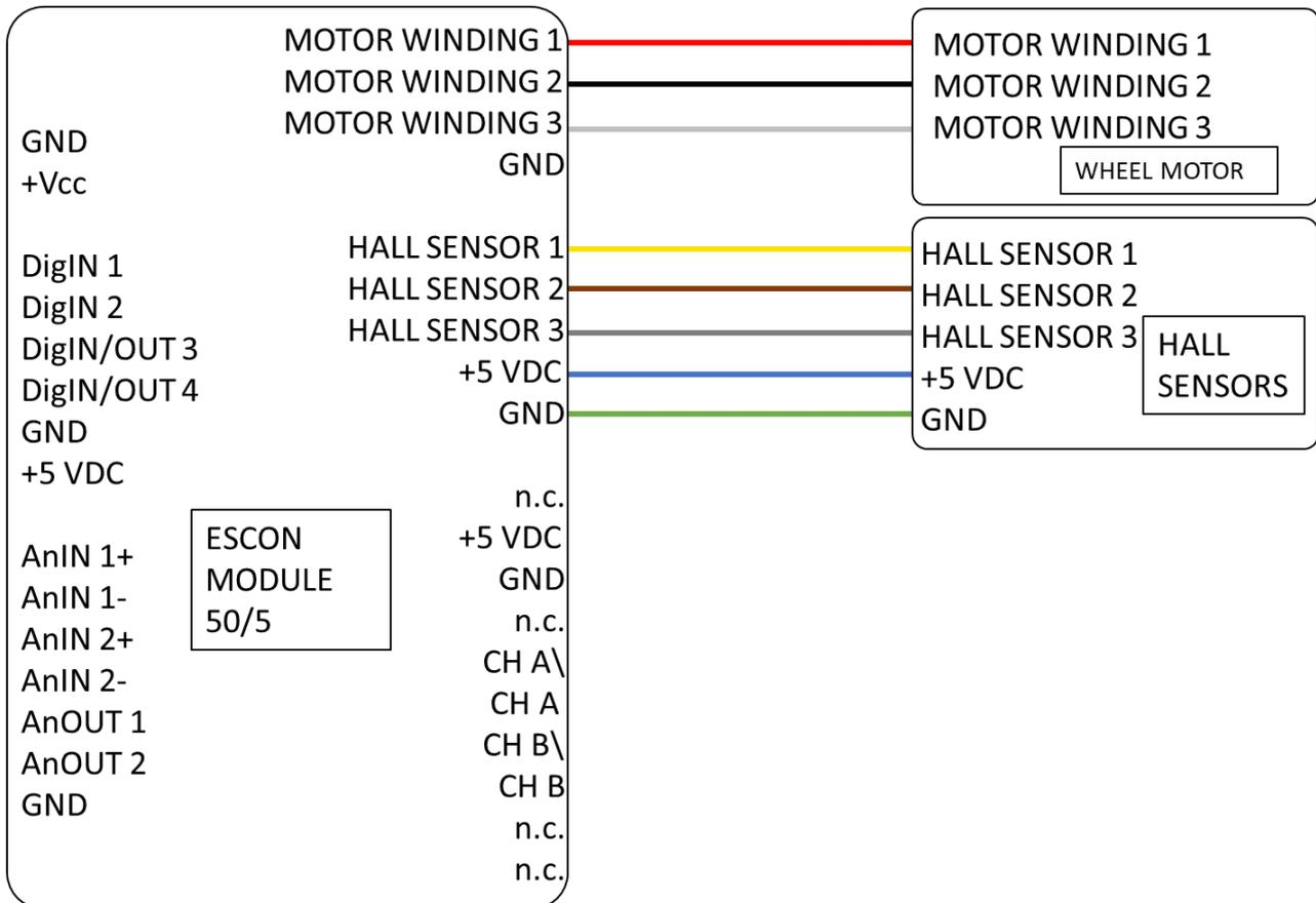
Figure 5.3 Escon module 50/5 -> EC frameless 45 flat connections
