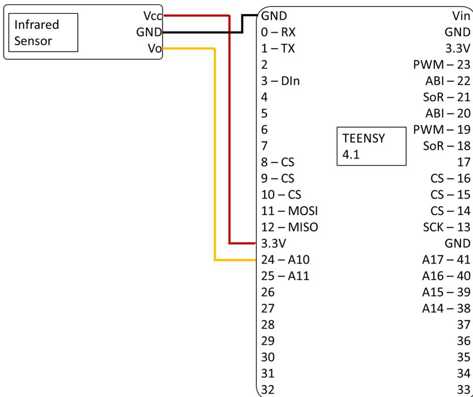
Figure 5.6 Infrared Sensors -> Teensy 4.1 connections
