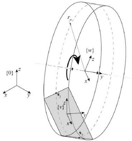
Figure 3.3 Definition of the reference frames for contact points
