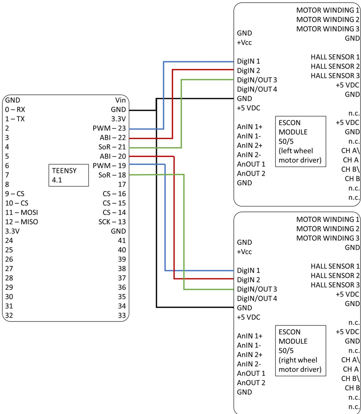
Figure 5.2 Teensy 4.1 -> Escon Module 50/5 connections
