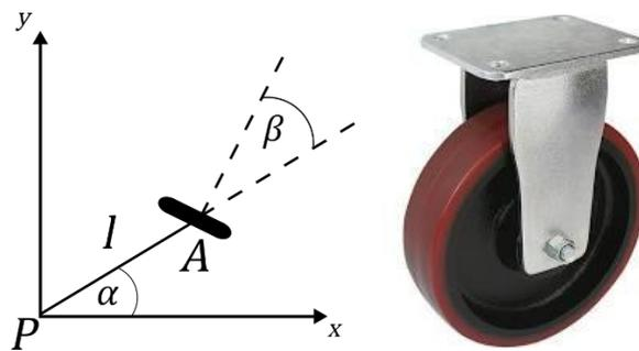
Figure 1.1 Fixed and Centered Orientable Wheel
