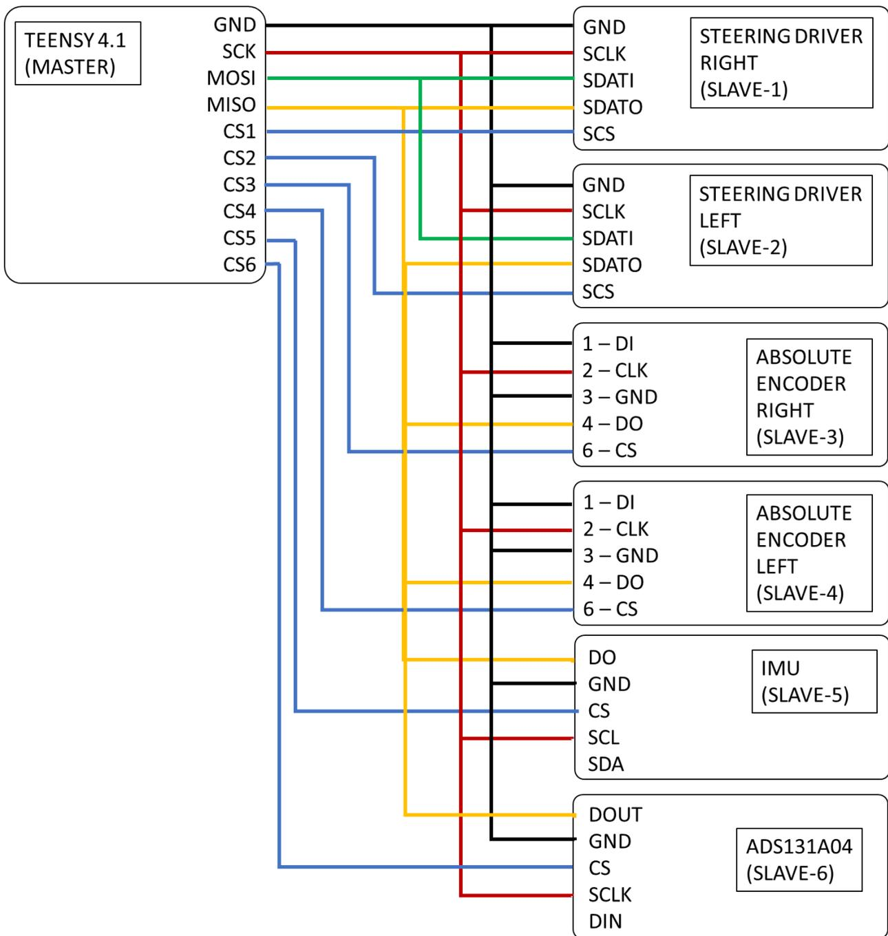
Figure 5.5 SPI Bus Connections
