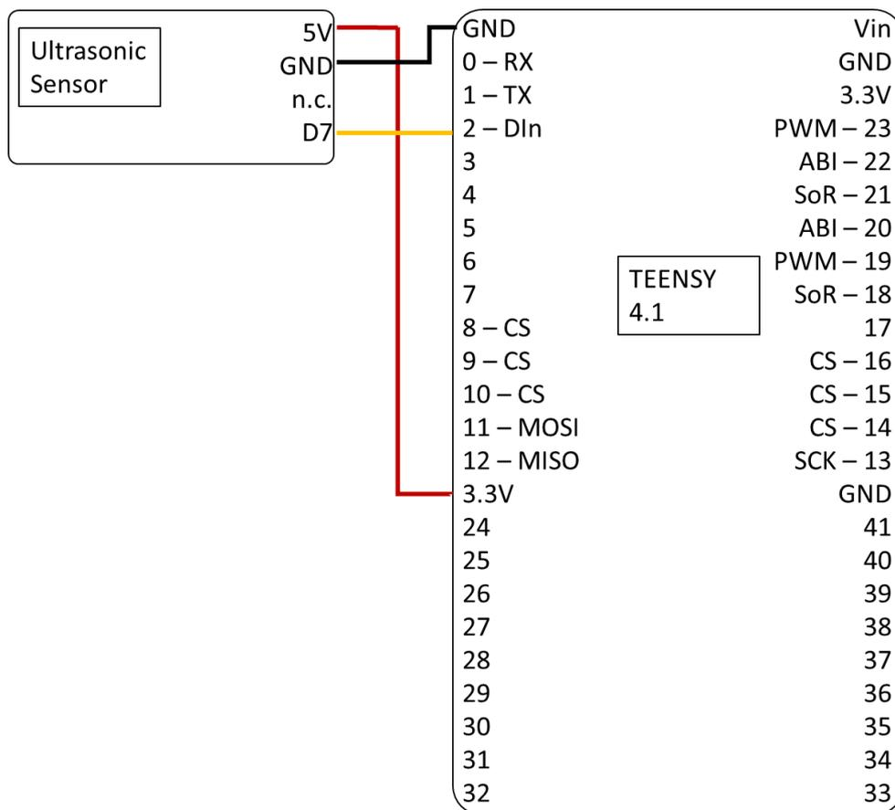
Figure 5.7 Ultrasonic sensors -> Teensy 4.1 connections
