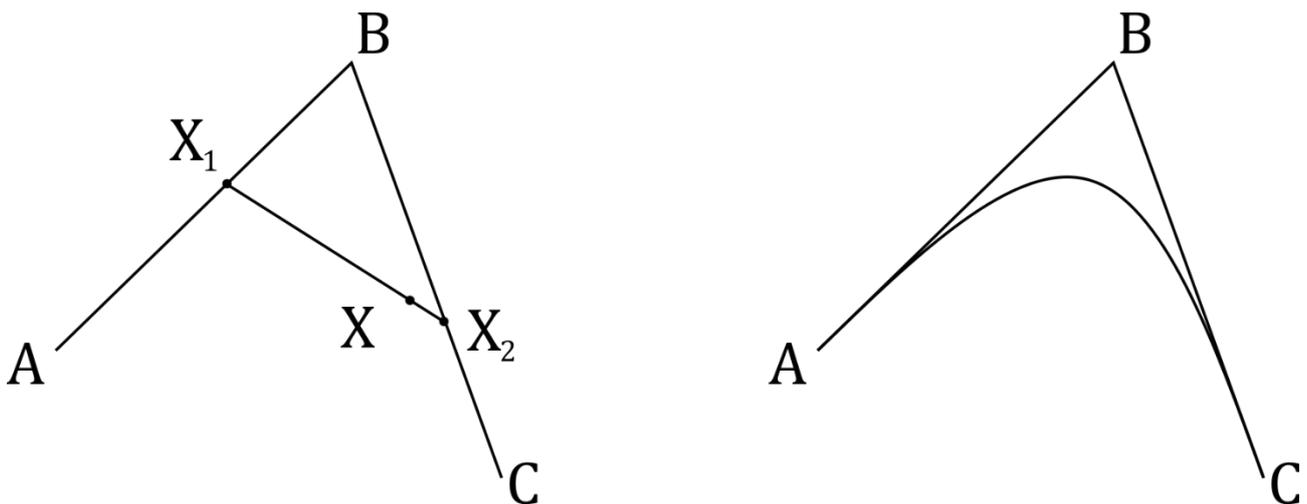
Figure 4.1 Bézier curve with one control point
