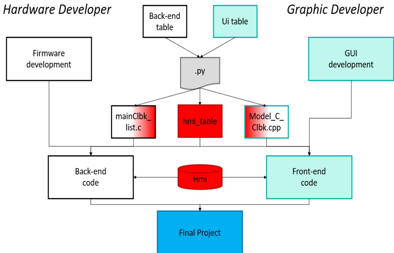
Figure 6.1: Main steps to implement a project with hmi.
