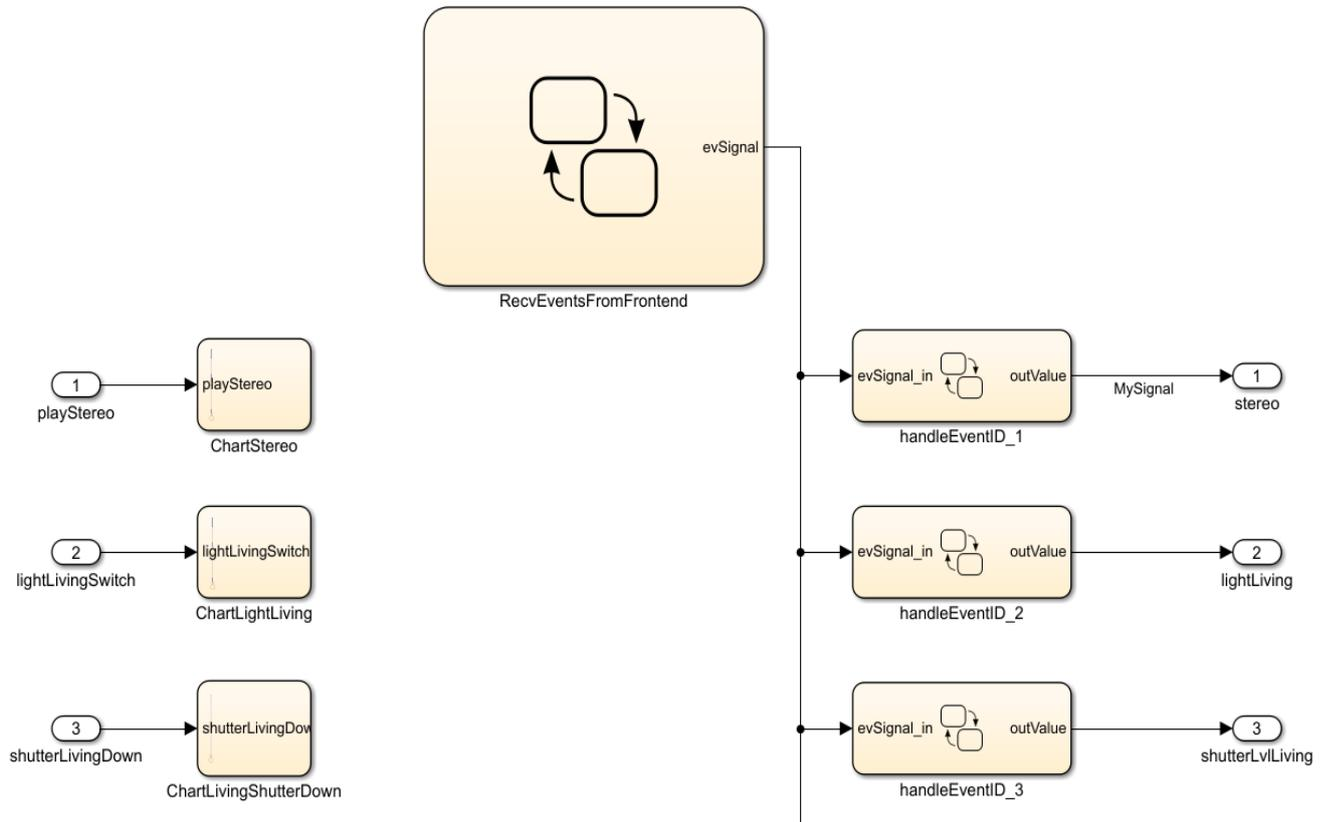
Figure 6.4: Internal structure of Simulink subsystem.
