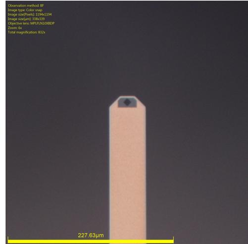
Figure 2.8: SSRM probe, zoom on the medium cantilever.
