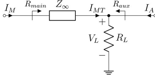
Figure 3.10: Circuitual equivalent of the output node
