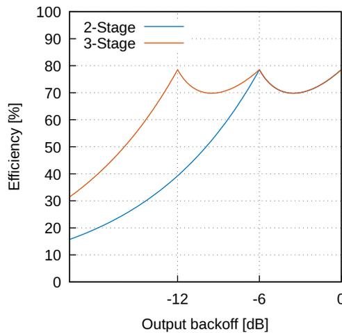
Figure 3.13: Efficiency of multi-stage DPAs
