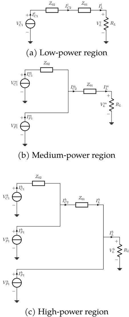
Figure 3.14: Equivalent circuits for a three-stage DPA
