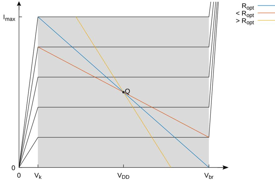
Figure 2.4: Load line behaviour
