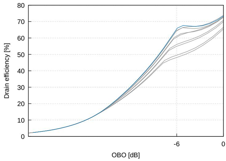
Figure 4.19: DPA drain efficiency – with swept  $f$
