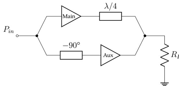
Figure 3.6: Block diagram of a Doherty amplifier
