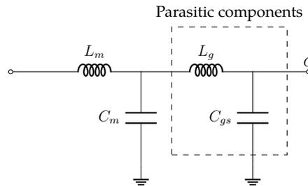
Figure 4.12: Lumped-element input matching network
