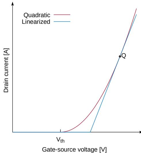
Figure 2.1: FET transconductance models
