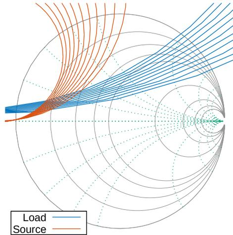
Figure 4.6: Load and source stability circles
