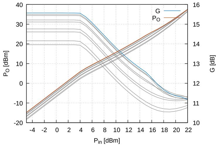
Figure 4.18: DPA output power and gain – with swept  $f$
