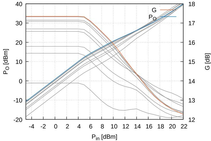
Figure 4.26: DPA output power and gain – with swept  $f$
