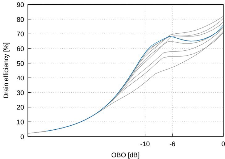
Figure 4.27: DPA drain efficiency – with swept  $f$
