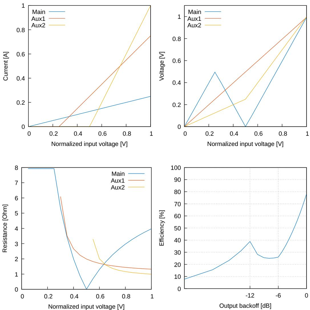
Figure 3.16: Device behaviour w/ linear Main current profile
