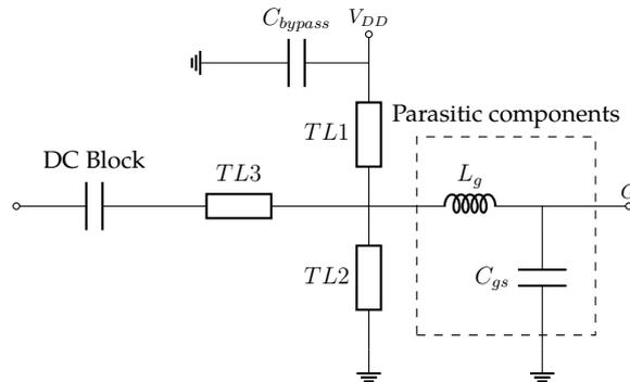
Figure 4.13: Distributed-element input matching network
