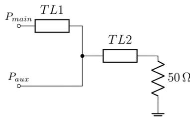
Figure 4.14: Distributed-element input matching network
