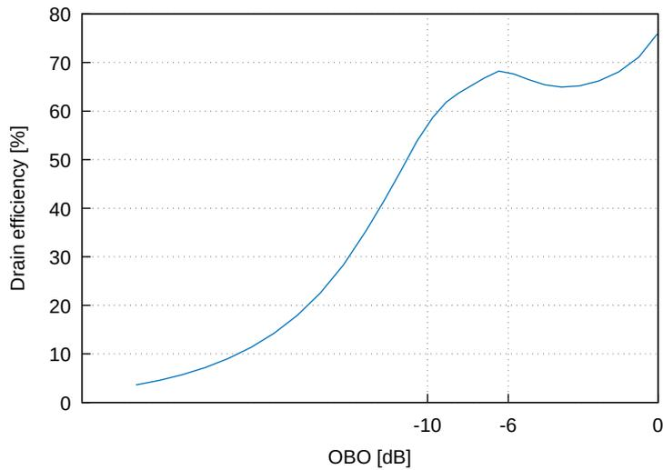
Figure 4.25: DPA drain efficiency
