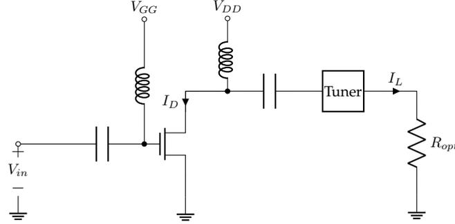
Figure 3.2: Tuned power amplifier
