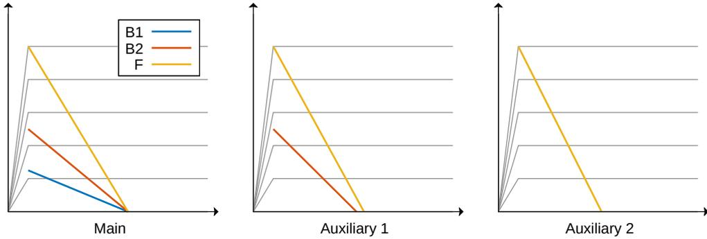
Figure 3.18: Load modulation for a three-stage DPA
