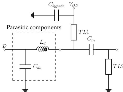
Figure 4.11: Distributed-element output matching network
