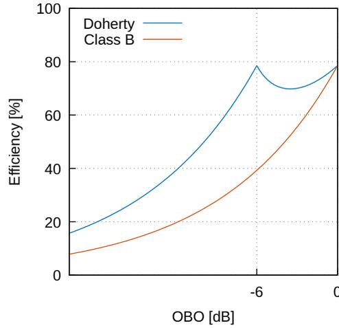
Figure 3.7: DPA drain efficiency
