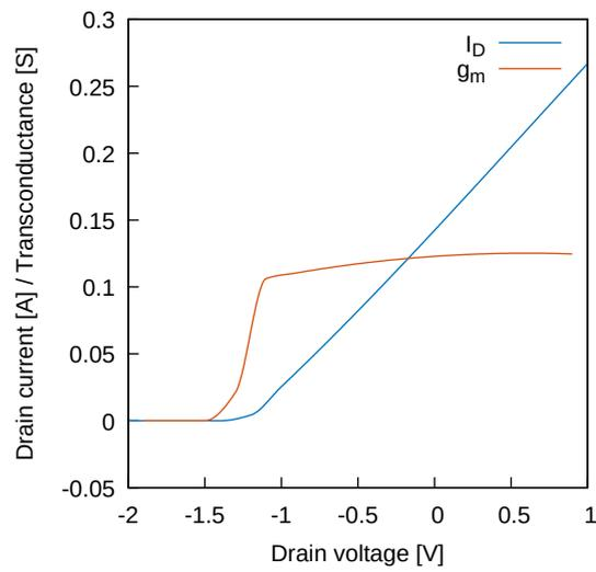
Figure 4.3: FET drain current behaviour
