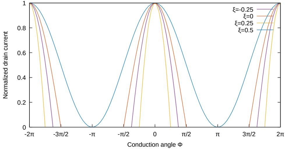
Figure 2.3: Drain current waveform for different values of  $\xi$
