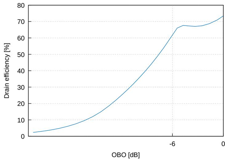
Figure 4.17: DPA drain efficiency
