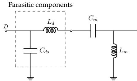
Figure 4.10: Lumped-element output matching network
