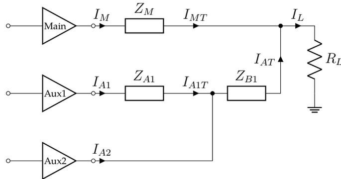
Figure 3.19: Annotated block scheme of the three-stage DPA
