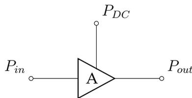
The signal amplification is done by a nonlinear component able to withstand large amounts of power. The typical choice for an active device is a Field Effect Transistor (FET) or Bipolar Junction Transistor (BJT), vacuum tubes were also widely used before the advent of the transistor and their use is now limited to niches where extremely high powers are handled. For the purpose of this work the use of a FET device is assumed.
