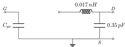
Figure 4.5: Simplified FET model for parasitics computation
