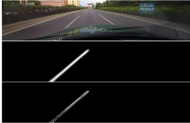
Figure 4.1: Example of feature extraction of left lane line. From top to bottom are the original image, the segmentation image, and the lane line extraction image.
