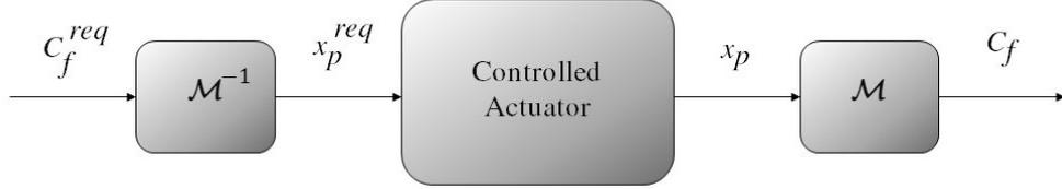
**Figure 3.4:** Controlled actuator structure. The feedback control system assures the tracking of a suitable reference signal  $x_p^{req}$  computed through the inversion of the map (3.5). While  $C_f^{req}$  is the requested clutch torque,  $C_f$  is the actual actuated torque.
