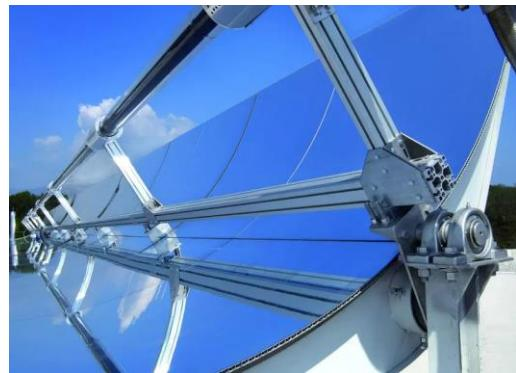
Fig. 4 Parabolic Trough Collectors
