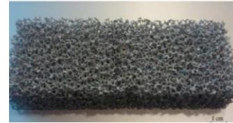
Fig. 16 Metallic porous blocks used in experiments on the cavity of a solid particle receiver.
