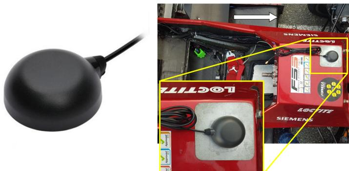
**Figure 3.8:** *GNSS antenna and its actual placement on the SC19D. The white arrow represents the direction of motion.*
