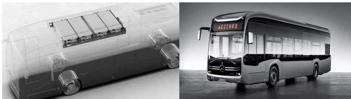
Figure 3.3: Mercedes-eCitaro-12m-264 kWh battery pack
