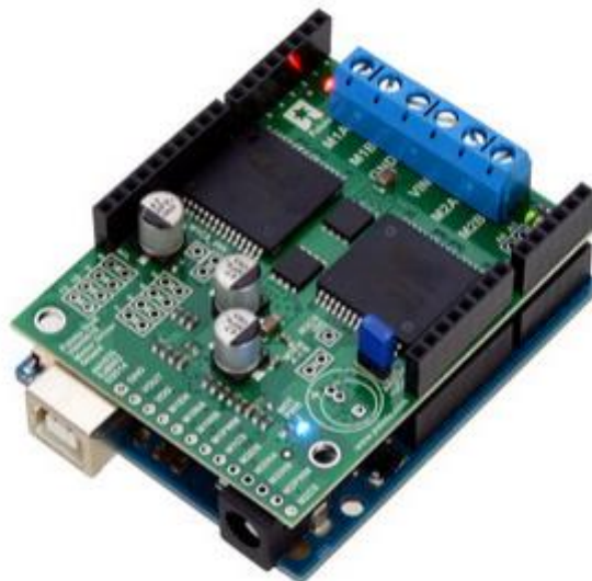
Figure 20 Dual VN5019 Motor Driver Shield assembled on Arduino Uno
