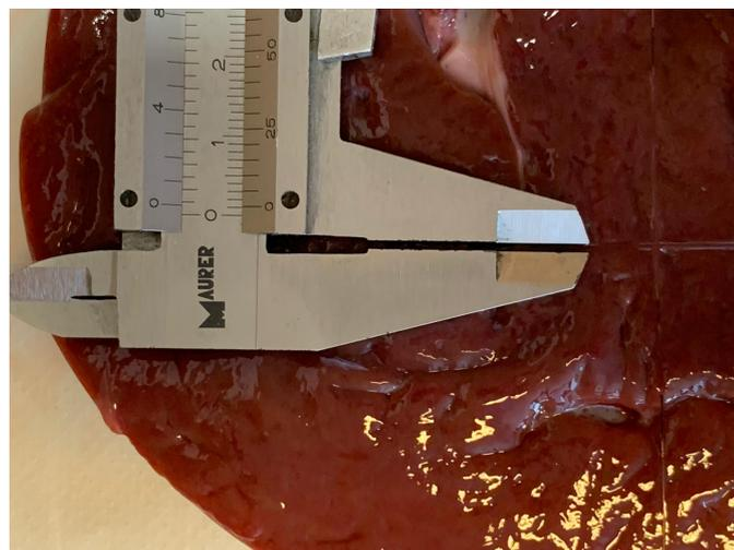
**Figure 7.5:** Zoom of the setup with the caliber.
