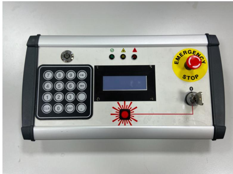
**Figure 7.2:** Complete Laser Unit. The keypad is used to insert the password, the power, the timer. When pushed, the red button below the display send the information of starting the emission. There is an emergency stop, a safety key and LEDs that help understanding laser status.
