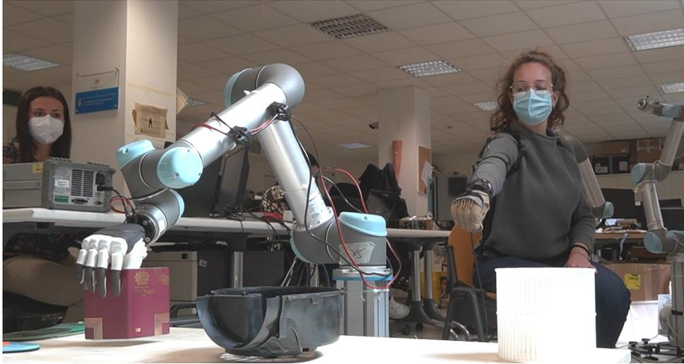
Figure 1.13: The teleoperated system developed during my thesis in action during a pick and place task.
