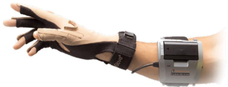
Figure 3.3: CyberGlove II motion capture data glove, instrumented with 18 high-accuracy joint-angle measurements [10].
