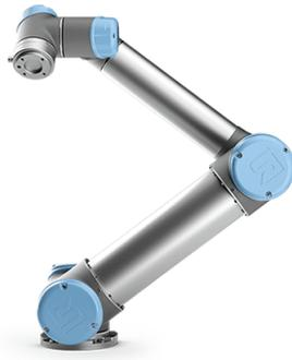
Figure 3.4: The 6-axis industrial robot (Universal Robot, model UR5)
