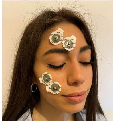
Figure 3.14: Electrodes placement on the mimics muscles.
