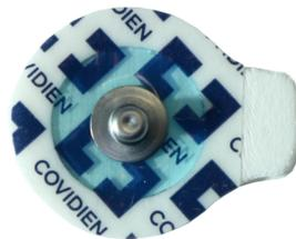
Figure 3.3: Electrodes used for sEMG acquisition.
