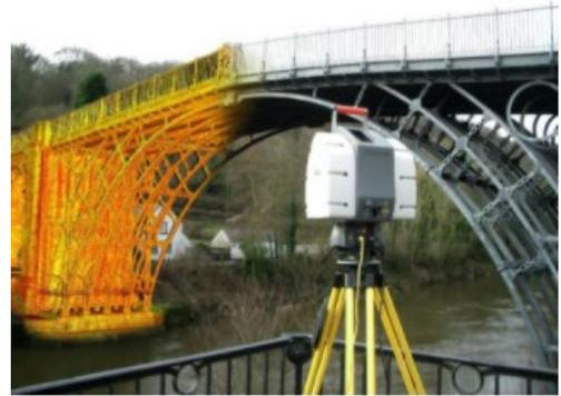
Figura 1.8: Scan to BIM
