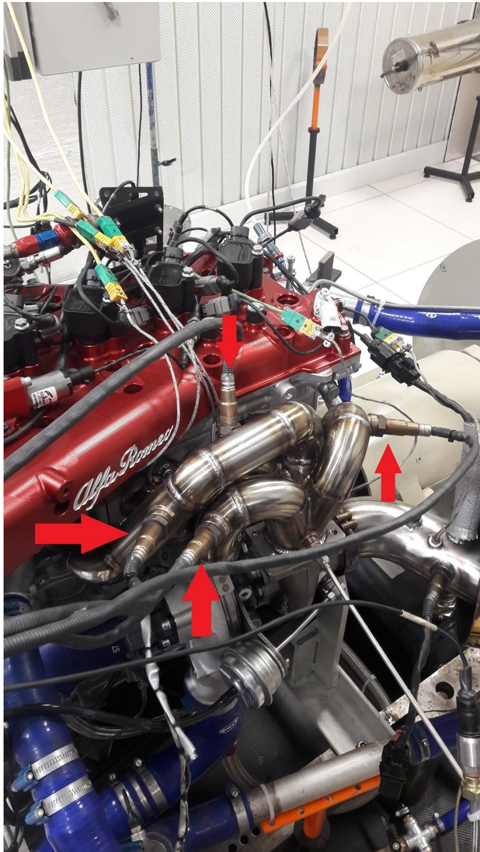
Figure 31. Lambda sensors on the ATM-AR-F3R EVO exhaust manifold.
