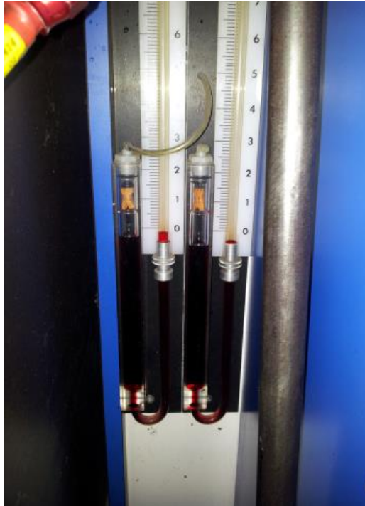
Figure 6. Pressure Gauge for the test pressure control.
