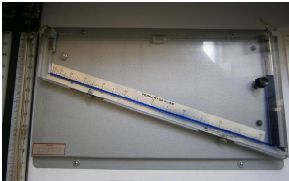
Figure 7. Pressure Gauge for the volumetric flow correction.
