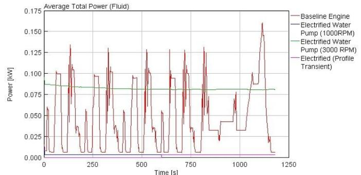
Figure 4. 2: Average Total Mechanical Power - NEDC
