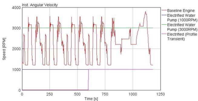
Figure 4. 1: Instant Angular Velocity - NEDC
