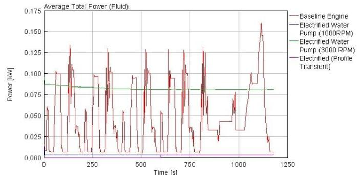
Figure 4. 2: Average Total Mechanical Power - NEDC
