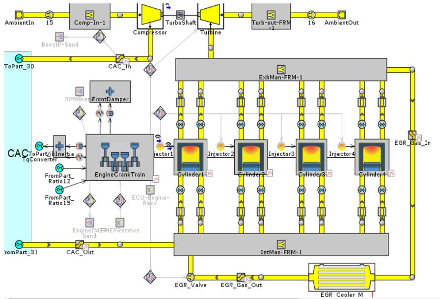
Figure 3. 3: Fast Running Engine Model (FRM) - Engine subassembly, Transient Warm-up Drive Cycle
