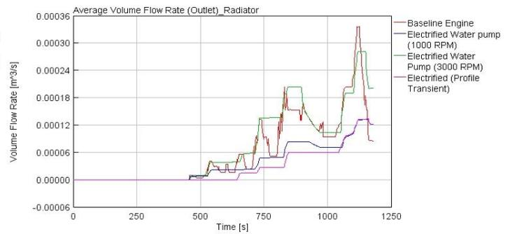
Figure 4. 12: Flow Rate (Radiator-Outlet) -NEDC
