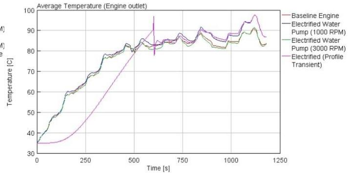
Figure 4. 8: Avg. Temp. (Engine Outlet)- NEDC
