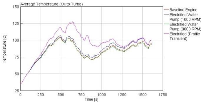
Figure 4. 17: Avg. Temp. (Oil to Turbo) -WLTC
