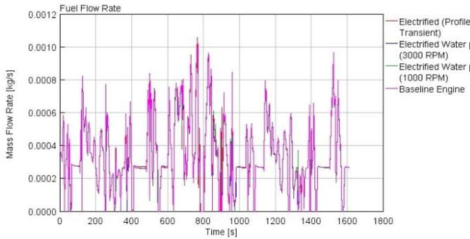
Figure 4. 25: Fuel Flow Rate -WLTC
