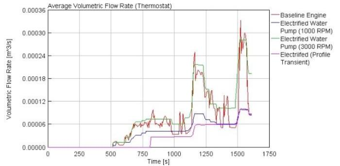
Figure 4. 26: Volume Flow Rate (Thermostat) -WLTC
