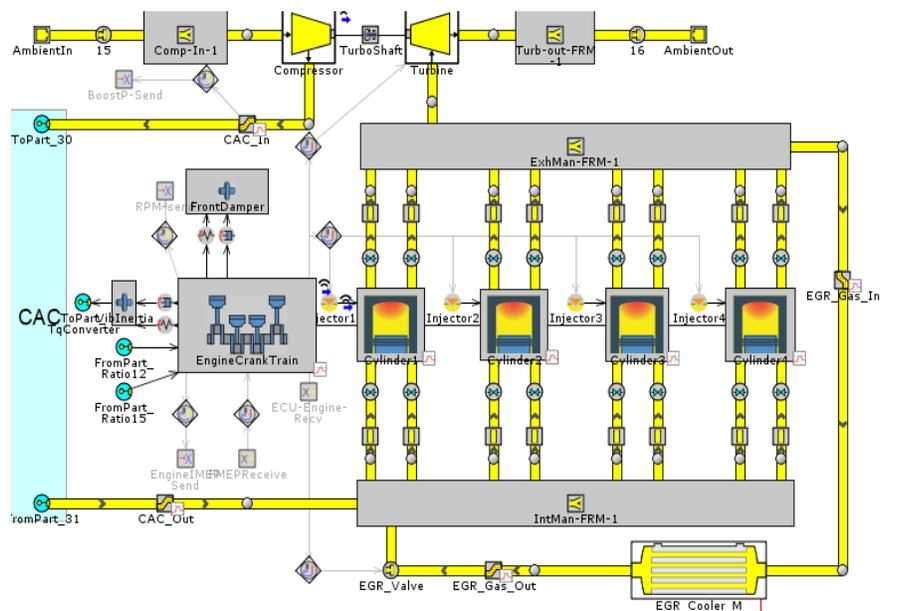
Figure 1. 1: Fast Running Engine Model (FRM) - Transient\_Warmup\_Drive\_Cycle\_Split\_Cooling.gtm
