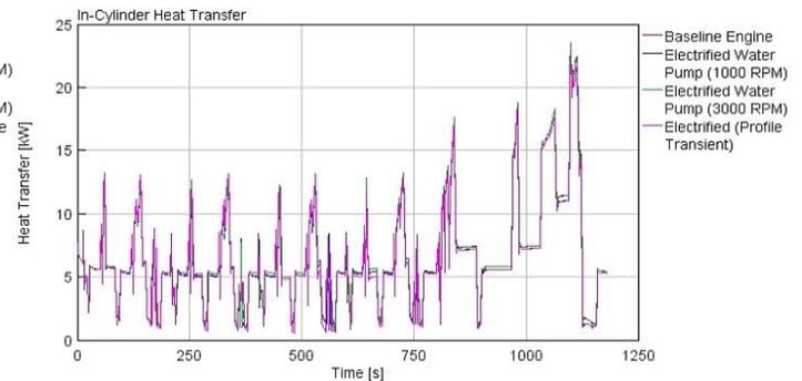
Figure 4. 10: In-cylinder Heat Transfer - NEDC
