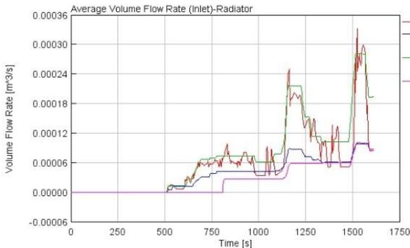
Figure 4. 23: Volume Flow Rate (Radiator Inlet) -WLTC
