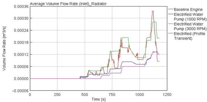
Figure 4. 11: Flow Rate (Radiator-inlet) -NEDC
