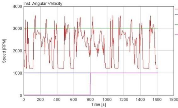
Figure 4. 15: Instant Angular Velocity -WLTC
