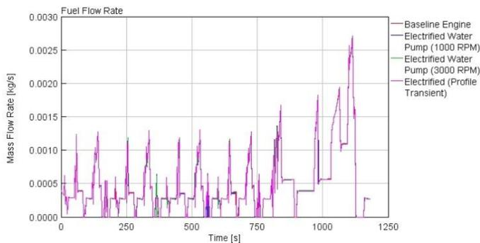
Figure 4. 13: Fuel Flow Rate - NEDC
