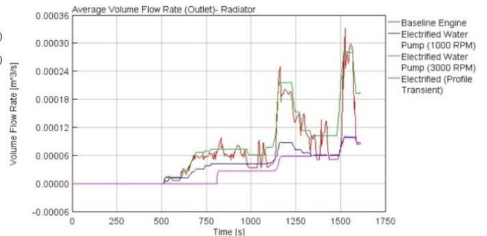
Figure 4. 24: Volume Flow Rate (Radiator Outlet) -WLTC
