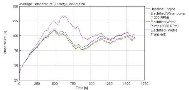
Figure 4. 18: Avg. Temp. (Block out Oil) -WLTC
