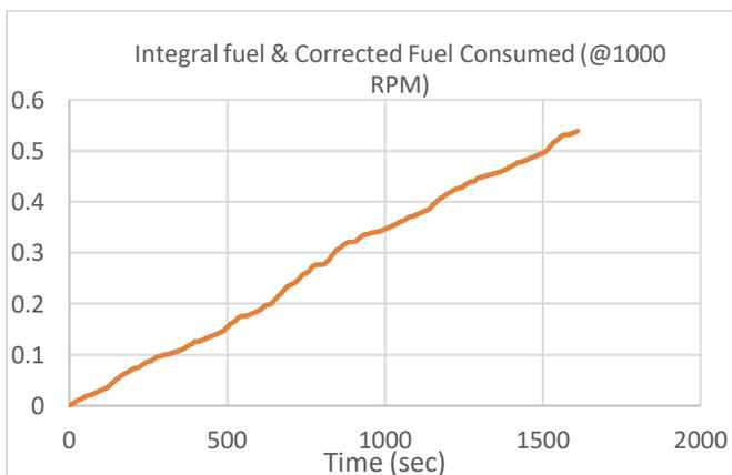
Figure 5. 7: Integral & Corrected Fuel Comparison- 1 (WLTC)
