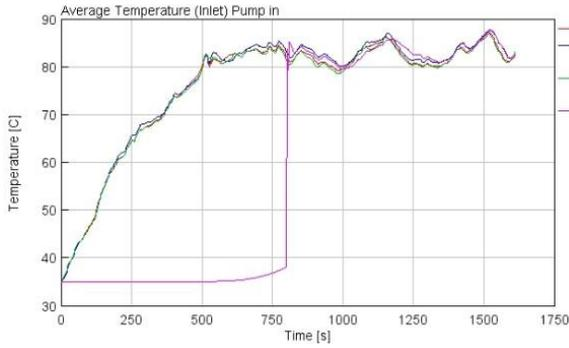
Figure 4. 19: Avg. Temp. (Water Pump-in) -WLTC
