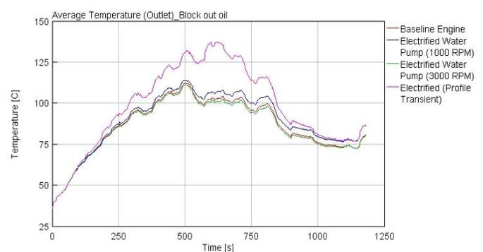
Figure 4. 4: Avg. Temp. (Block out Oil) – NEDC
