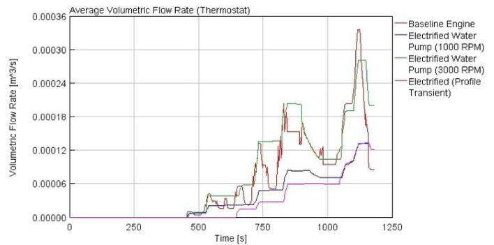
Figure 4. 14: Volume Flow Rate (Thermostat) –NEDC
