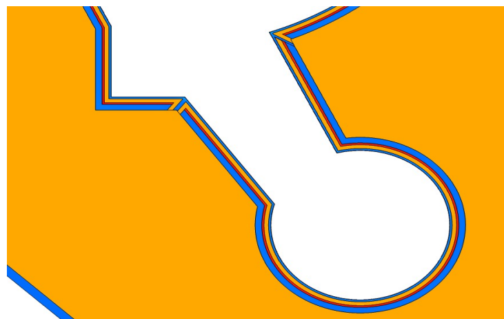
Figure 2.5 - Leg and foot region for ARC. Outlet model from vacuum vessel to tank. FLiBe is orange, Inconel blue, Beryllium red. Tungsten is darker blue, but as 1 mm thin layer it cannot be seen.
