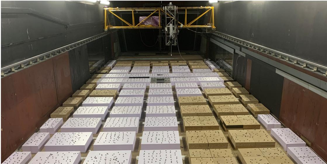
Figure 3.2: Street network inside the wind tunnel
