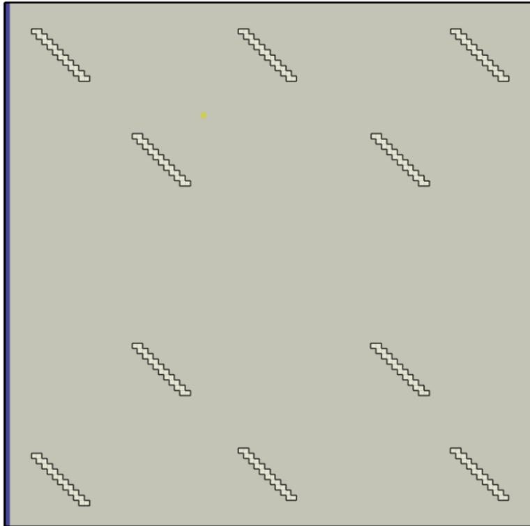
*Figure 33 Condition with 10 fractures inclined 45 ° of 100 meters*
