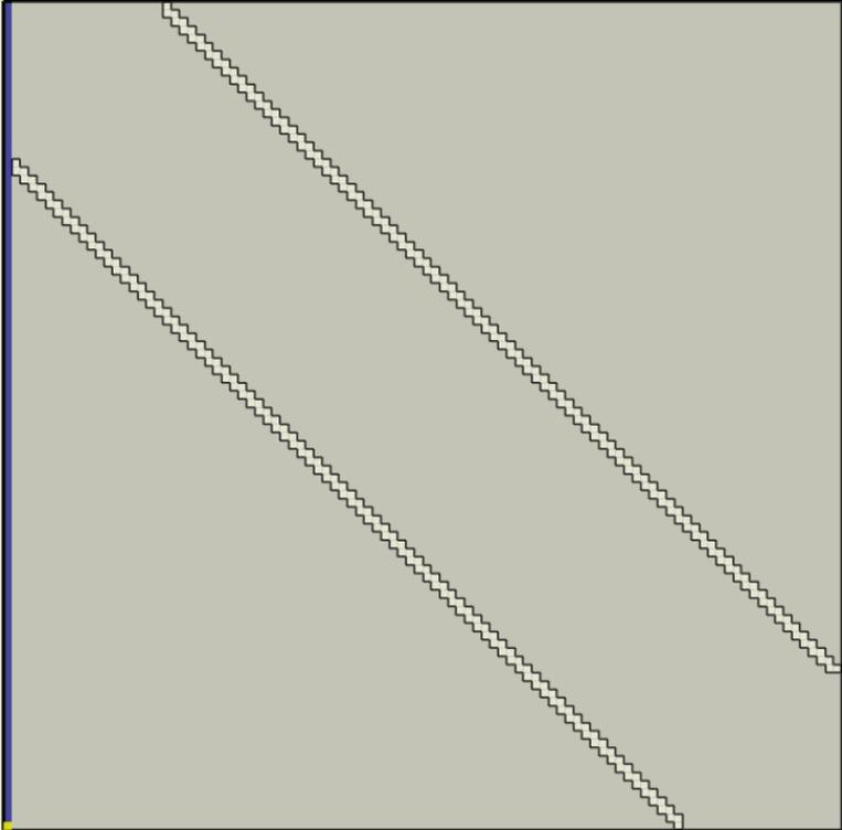
*Figure 26 Condition with 2 fractures inclined at 45 ° of 1000 meters*
