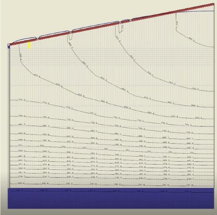
Figure 43 Error in the over-raising of the starting Hydraulic head
