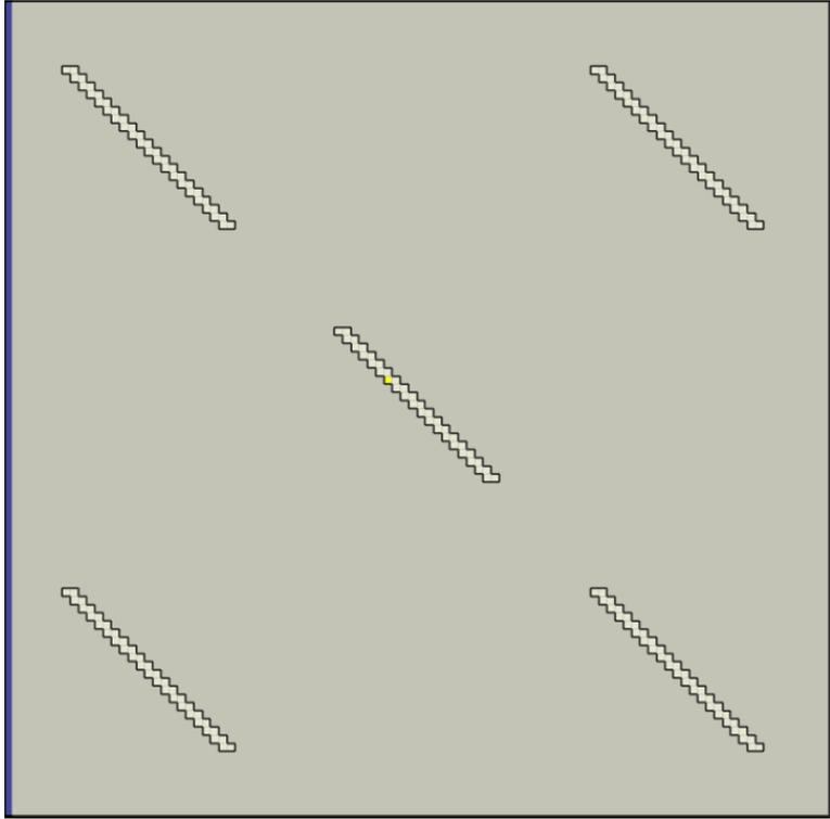
*Figure 29 Condition with 5 fractures inclined at 45 ° of 200 meters*
