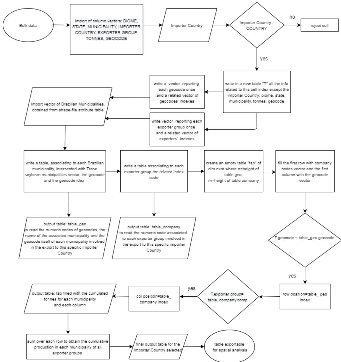
Figure 3.1.3: Flow chart representing the algorithm for data elaboration and extraction
