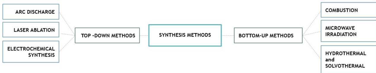
Figure 2 Synthetic routes for carbon dots production
