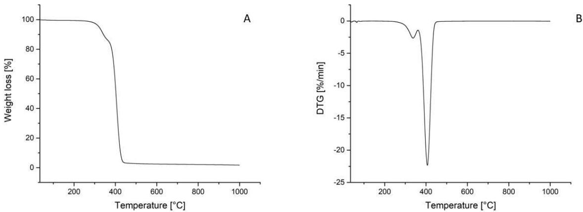
Figure 31 TGA analysis for EM-26: (A) weight loss (B) DTG.
