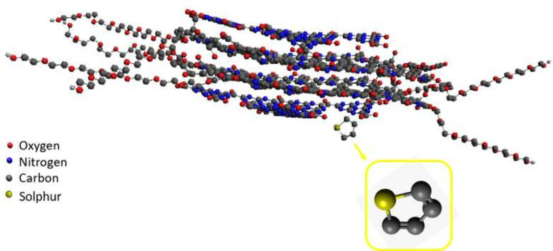
*Figure 42 First possible configuration for PEG-containing Carbon Dots loaded with one molecule of thiophene.*
