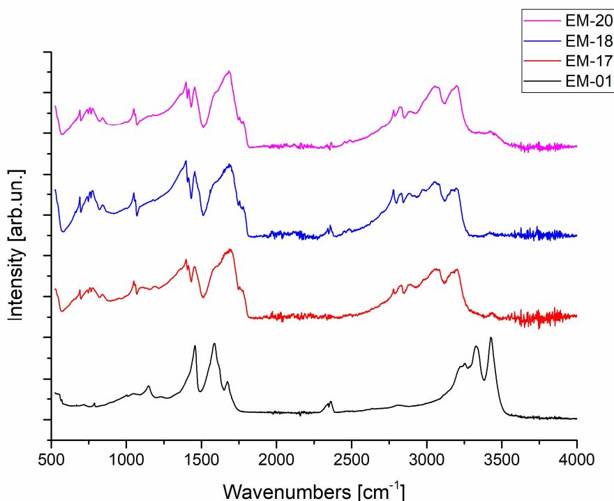
Figure 17 The IR spectra of the precursor EM-01 and the products: EM-17, EM-18, EM-20.
