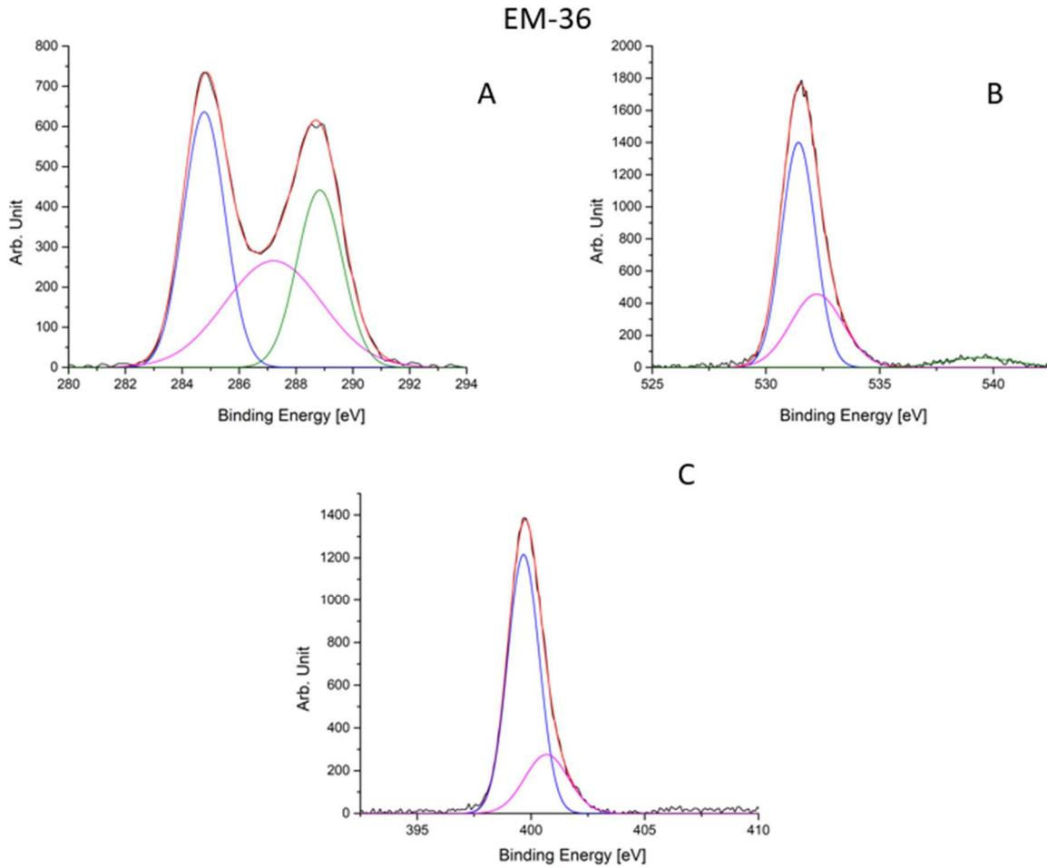
Figure 33 XPS results for EM-36 (A) Carbon, (B) Oxygen, (C) Nitrogen.
