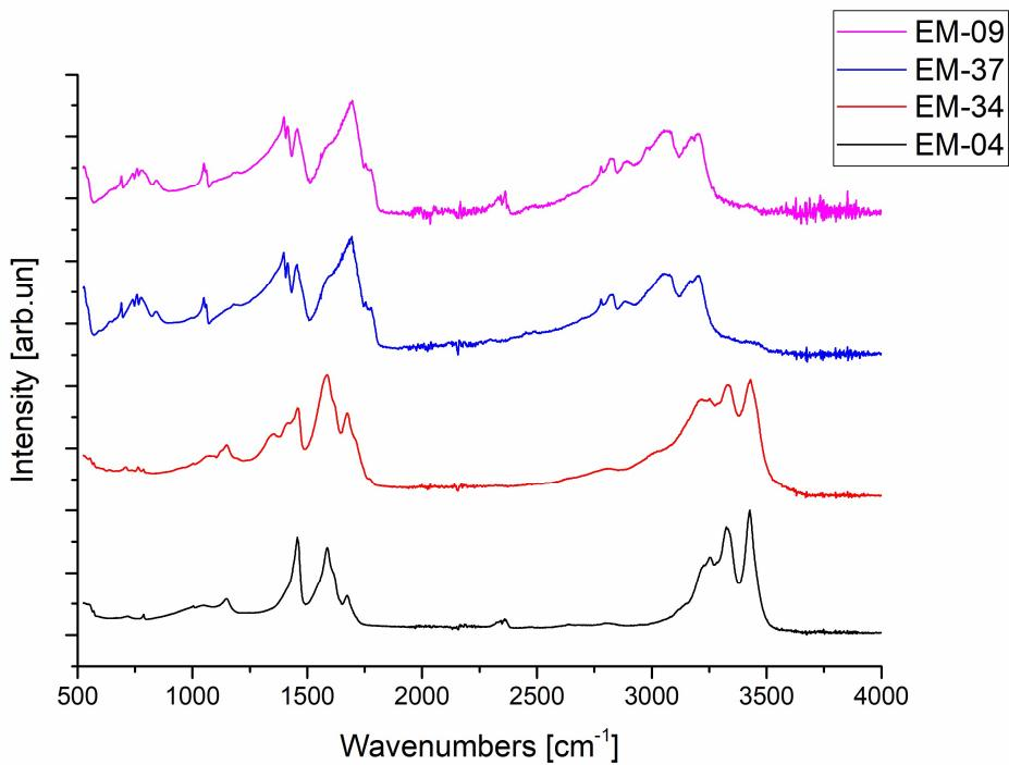
Figure 18 The IR spectra for the synthesis at 350 °C, 450 °C and 550 °C for ten minutes of the precursor EM-04.
