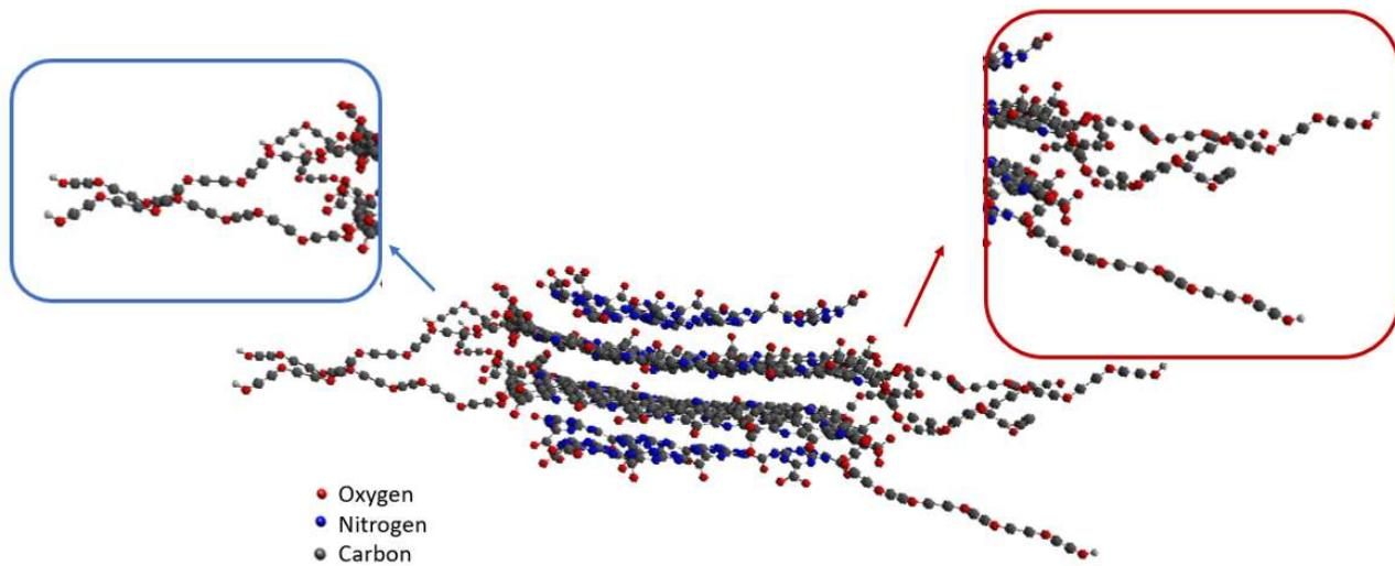
Figure 38 Carbon Dot containing PEG structure's simulation.
