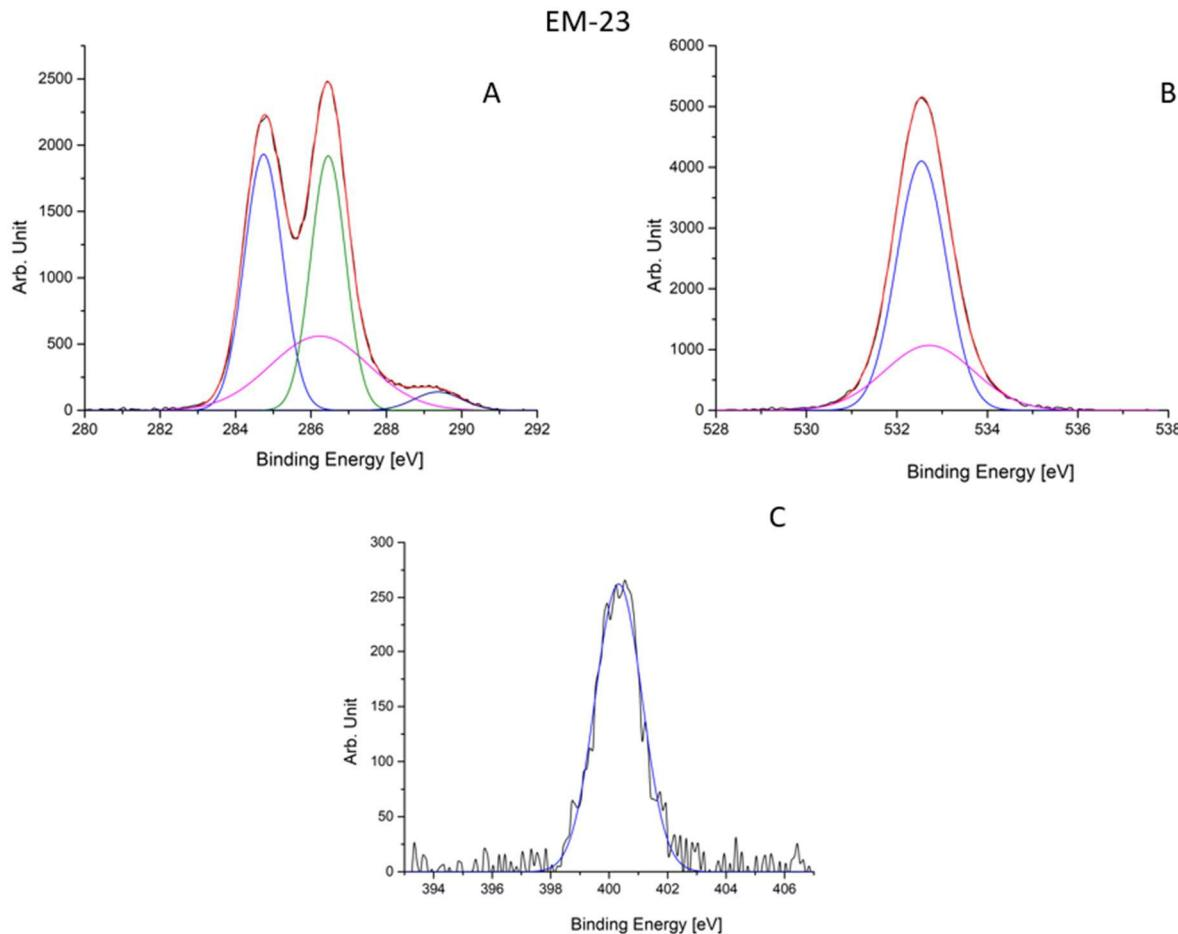
Figure 34 XPS results for EM-23, (A) Carbon, (B) Oxygen, (C) Nitrogen.
