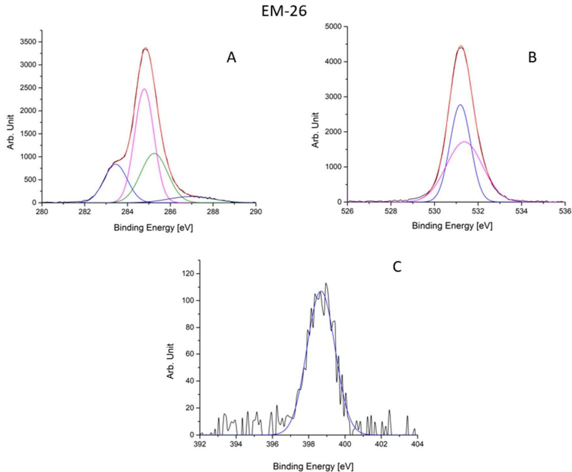
Figure 35 XPS results for EM-26, (A) Carbon, (B) Oxygen, (C) Nitrogen.
