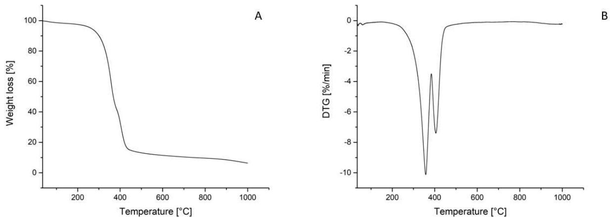
Figure 30 TGA analysis for EM-23: (A) weight loss (B) DTG.
