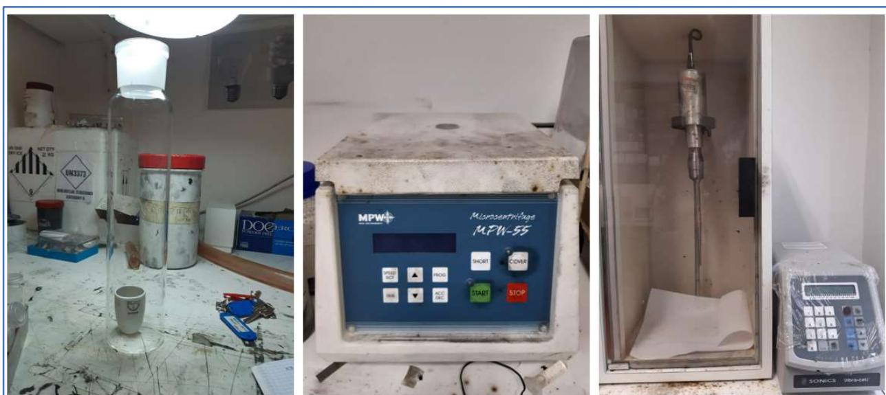
Figure 7 Pyrex tubular reactor, Microcentrifuge MPW-55, Vibra Cell Sonicator.
