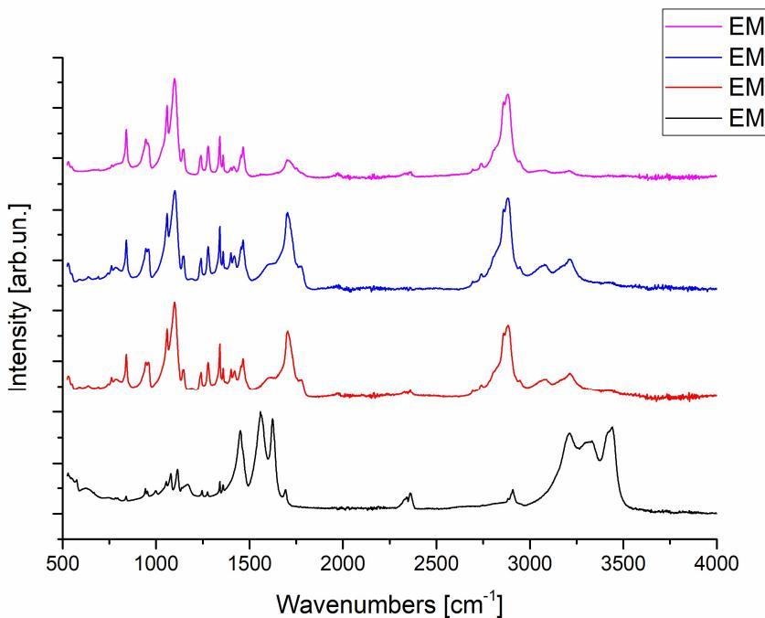
Figure 26 The IR spectra of the products for the syntheses of EM-06 at 550 °C with different reaction times.
