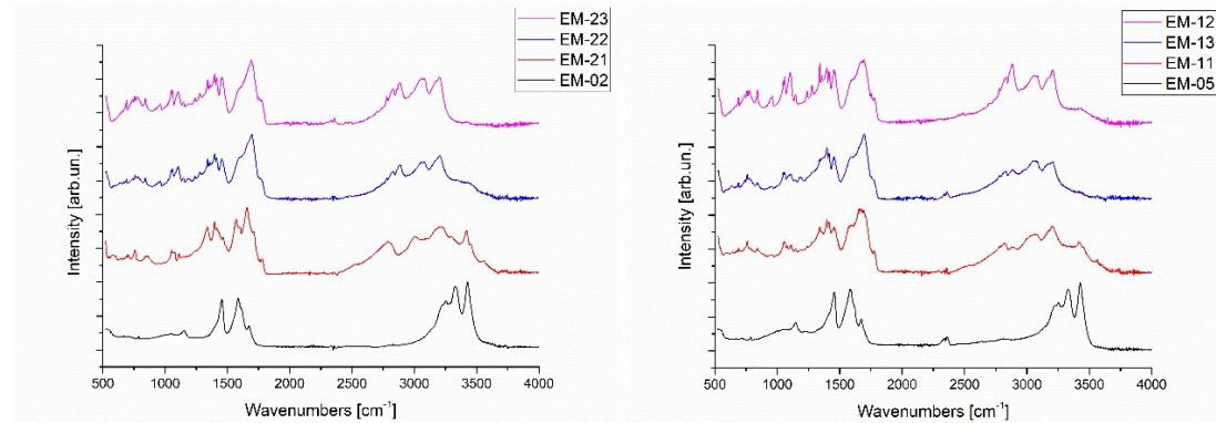
Figure 22 The IR spectra of the precursor EM-02 with its products at  $550\text{ }^{\circ}\text{C}$  on the left. The IR spectra of the precursor EM-05 with its products at  $550\text{ }^{\circ}\text{C}$  on the right.
