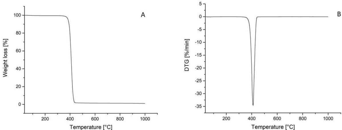
Figure 29 TGA analysis of PEG: (A) weight loss (B) DTG.
