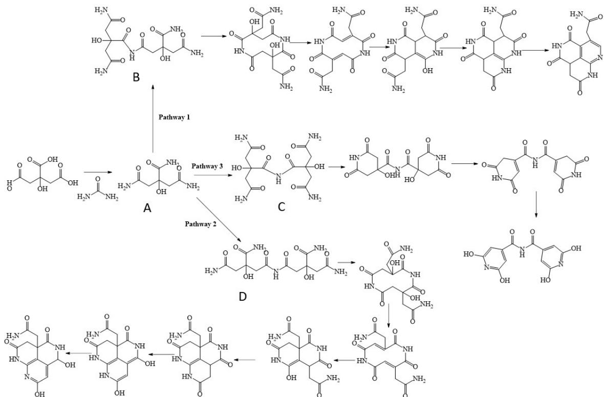
Figure 11 Chemical pathways during the thermal reaction of Citric Acid and Urea.
