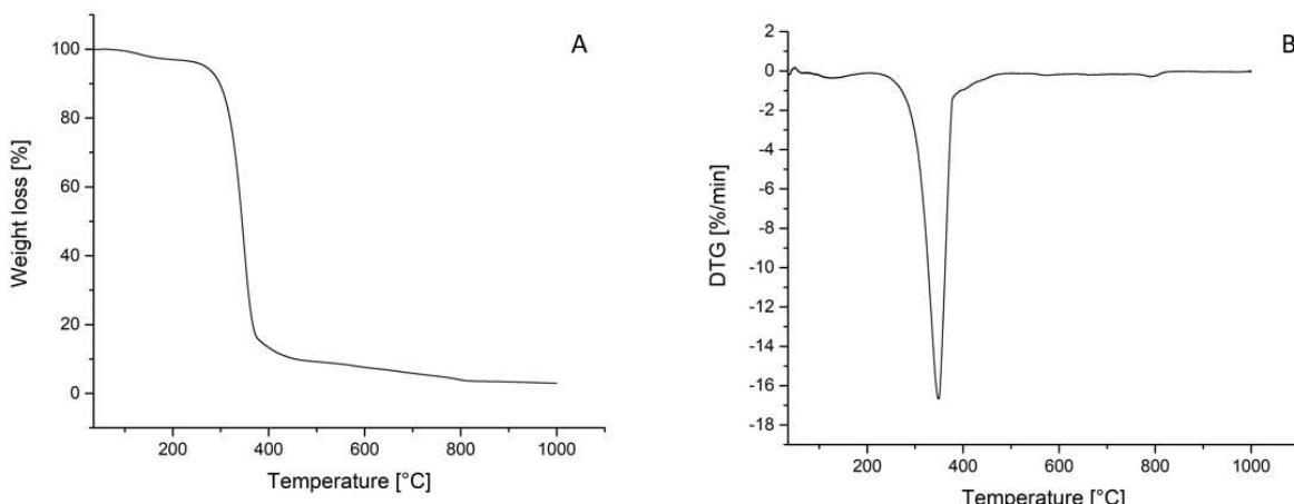
Figure 27 TGA analysis for EM-18: (A) weight loss (B) DTG.
