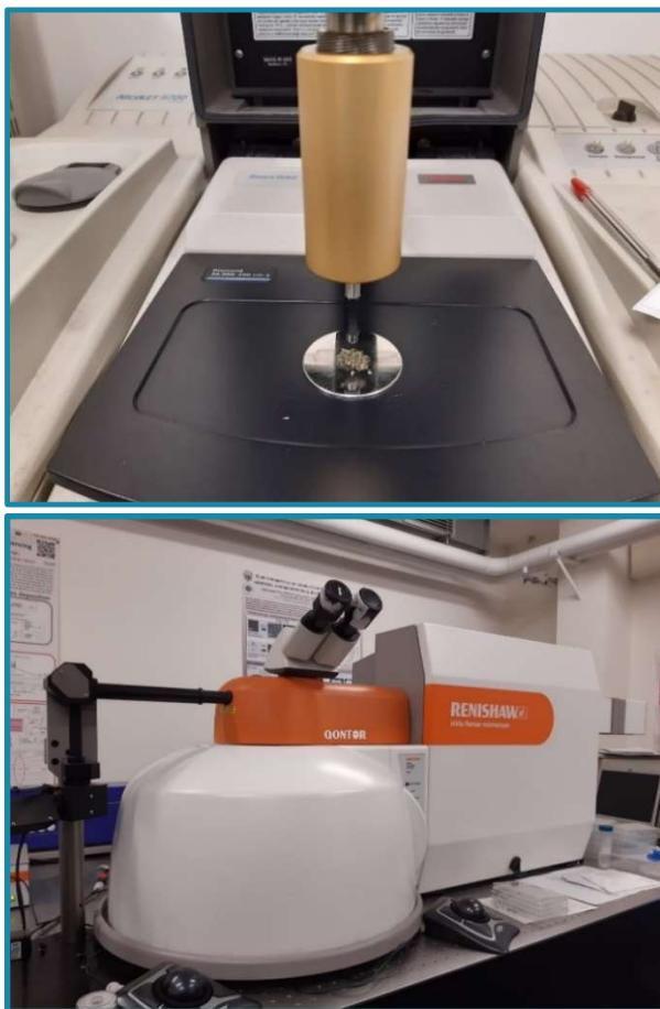
Figure 10 Infrared Spectroscopy and RAMAN equipment.
