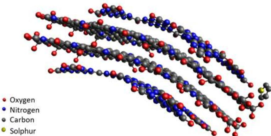
*Figure 39 Simulation of a Carbon Dot loaded with one molecule of thiophene.*
