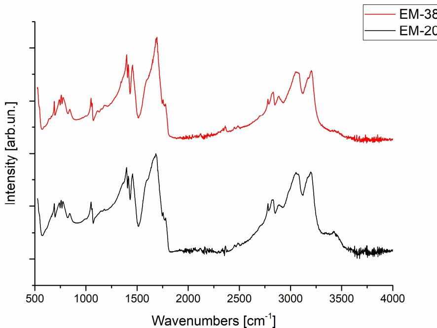
Figure 19 The IR spectra of the products EM-20 and EM-38 with 10 minutes and 15 minutes reaction times.
