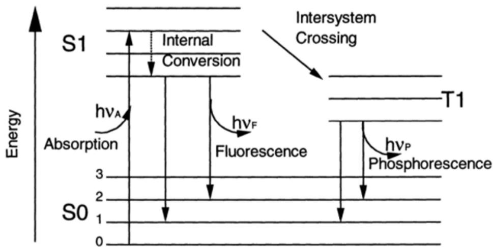
Figure 4 Photoluminescence mechanism scheme.
