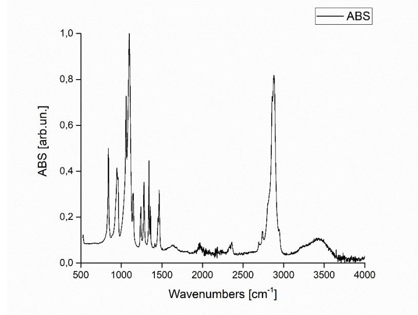
Figure 20 The IR spectrum for the reagent PEG.
