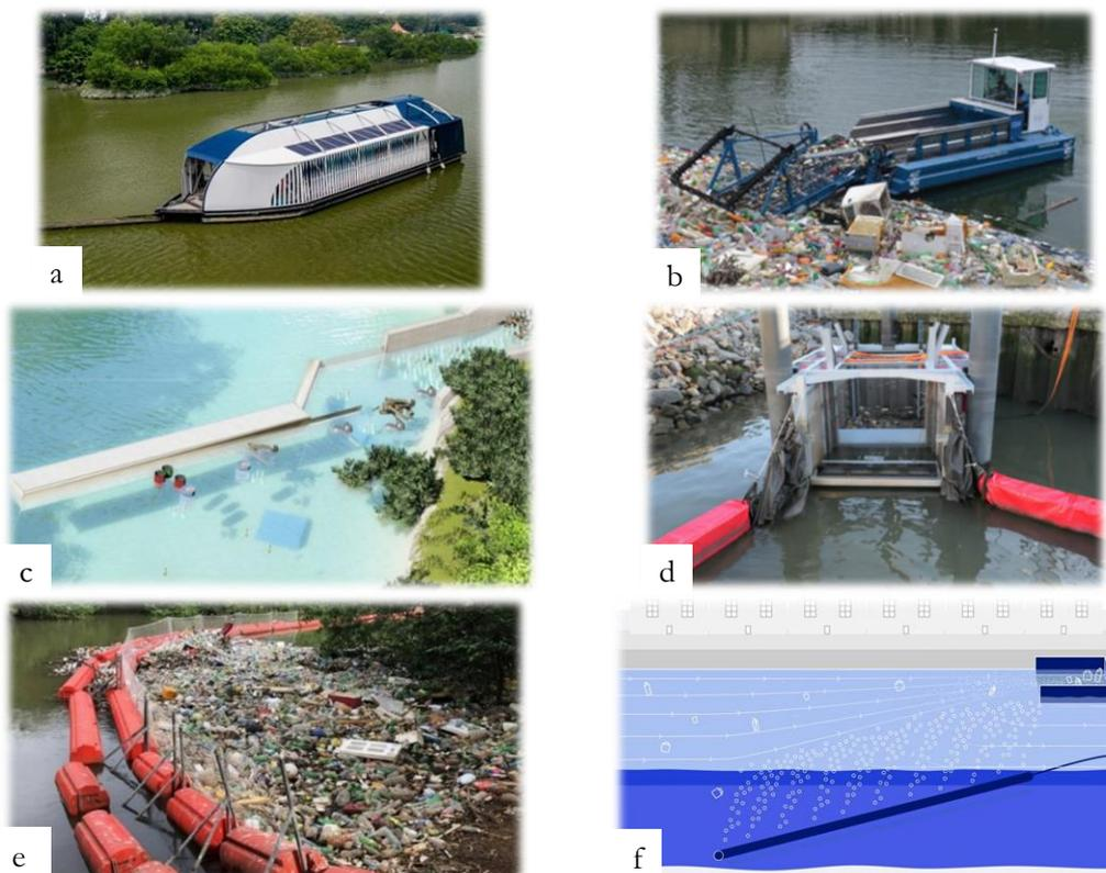
**Figura I.4** - a) *TheOceanCleanup Interceptor*; b) *CollectiX*; c) *Sea Defence Solutions*; d) *Allseas river plastics removal system*; e) *B.O.B. Litter Trap*, installato da *Marea Verde* con la *Clean Currents Coalition*; f) *The Great Bubble Barrier*
