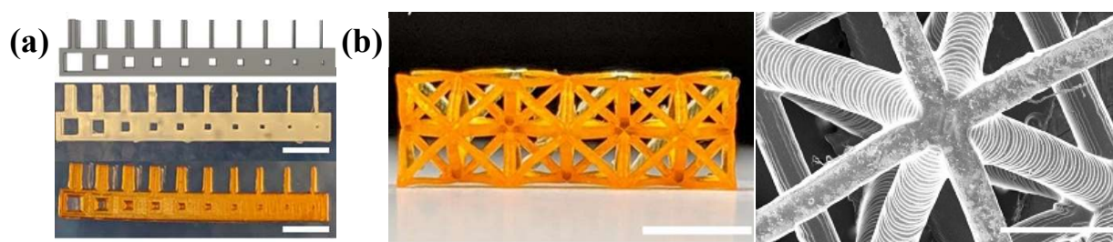
Figure 3.19 (a) From top to bottom, comparison of the original CAD, printed commercial resin, and resin based on methacrylated bovine serum albumin. Scale bars: 5 mm. (b) Optical image (left) and SEM image (right) of lattice structure made of resin containing methacrylated bovine serum albumin; in the SEM image 50 \mu\text{m} layer heights are visible. Scale bars: 5 mm (left), 1 mm (right). [89]
