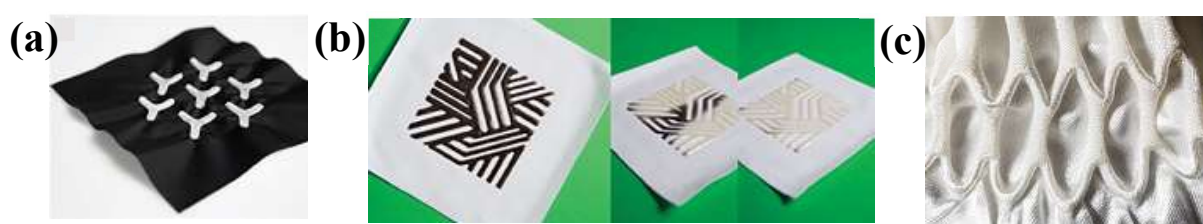
Figure 3.10 (a) Refractive structures from an ink based on cellulose acetate. (b) Thermoresponsive structures from an ink based on acetoxypopyl cellulose. (c) Structures printed using cellulose dissolved in ionic liquid for smocking effect. [63]
