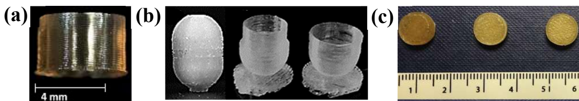
Figure 3.5 (a) Hollow cylindrical implant of ethylcellulose in side view (outer diameter of 5 mm, inner diameter of 3 mm). [39] (b) Capsular device made of hydroxypropyl cellulose (diameter of 7 mm, height of 13 mm). [40] (c) Printlets (10 mm in diameter, 3.6 mm in height) incorporating 5% paracetamol: increasing hydroxypropyl methylcellulose acetate succinate grade from left. [42]
