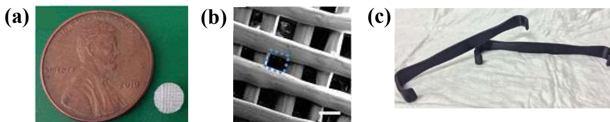
Figure 3.3 (a) PLA cylindrical scaffold compared to a cent. [32] (b) SEM image of porous PLA scaffold. The blue square shows 200 µm pores. [33] (c) Two FDM printed surgical instrument prototypes made of PLA. [34] (The scale bar indicates 200 µm.)
