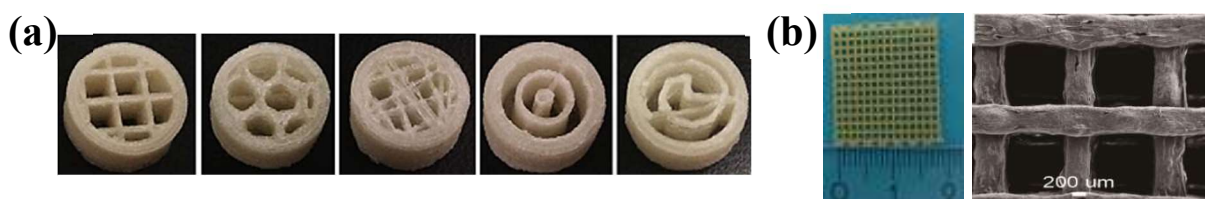
Figure 3.6 (a) Printed tablets of ethylcellulose and hydroxypropyl methylcellulose blend (12.0 mm diameter, 7.0 mm height, 200 \mu\text{m} layer height). [44] (b) Printed scaffold (20 mm x 20 mm x 2 mm) and top view SEM image, referred to blend ratio of 20:80 in weight of galactoglucomannane and PLA. [46]
