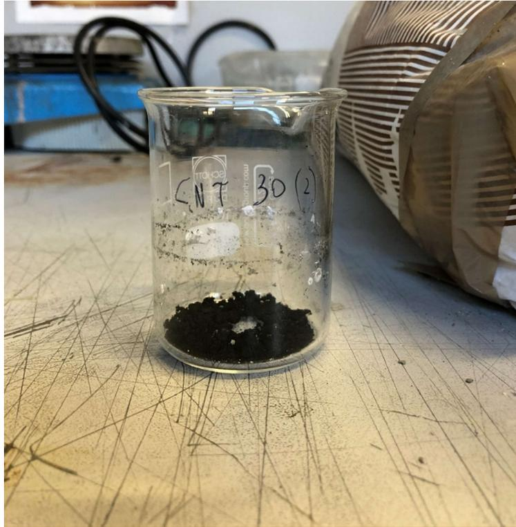
*Figure 27. Result of 30 minutes of sonication in the sulfonitric acid solution for CNTs*
