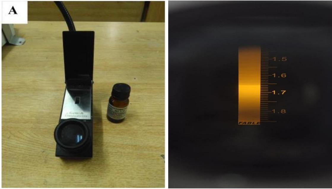
**Fig. 5.1.** (A) Standard Refractometer with R.I fluid (Di-iodomethane); (B) Termination of the shadow of refractive Index showing the value of 1.660.
