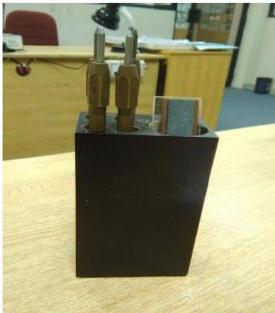
Fig. 5.3. Standard hardness pencils ranging from 2 to 9 hardness.
