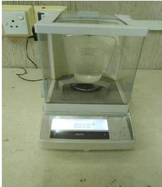
Fig. 5.2. Standard Hydrostatic weighing-Machine for measuring specific gravity.
