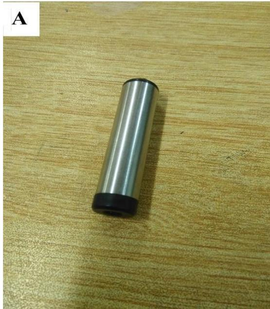
Fig. 5.5. Standard diffraction grating spectroscope
