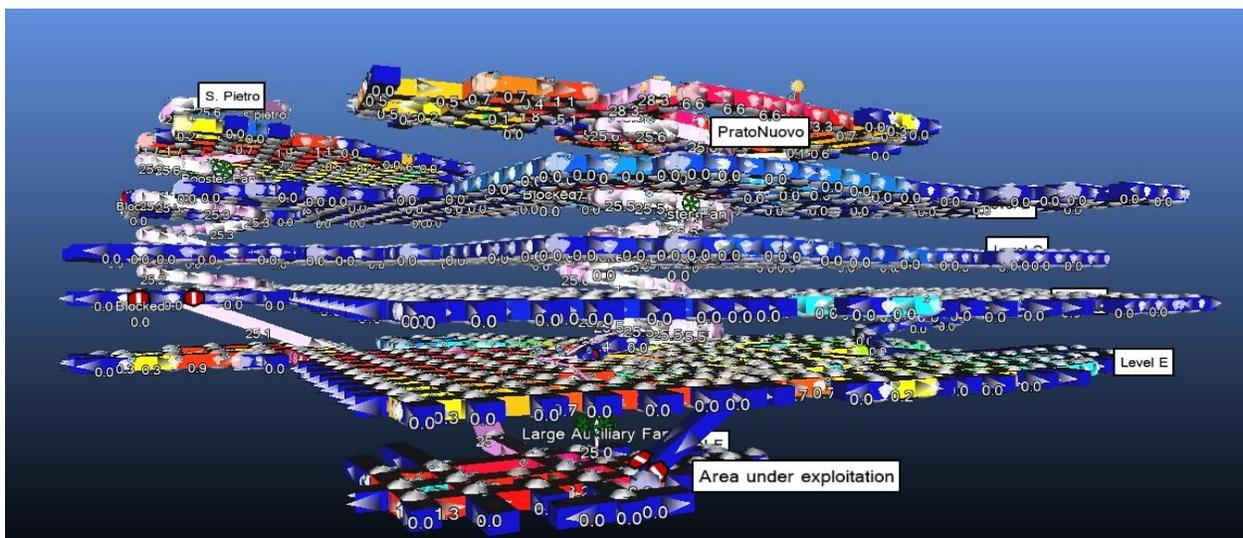
Figure 8.31: The amount of airflows inside different airways in the final solution.
