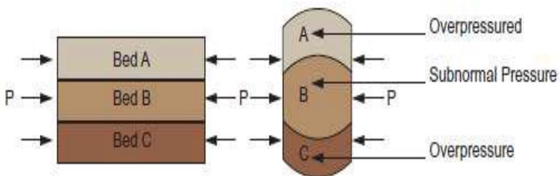
Figure 1.10 (The different layout of the beds ) [7]
