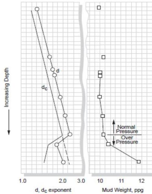
Figure 2.2 The detection of the geo-pressure by using both the D and  $D_c$  exponents[36]
