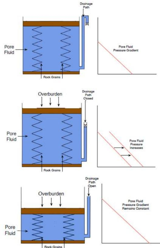
Figure 1.9 (Overpressure Generation Mechanism)[20]
