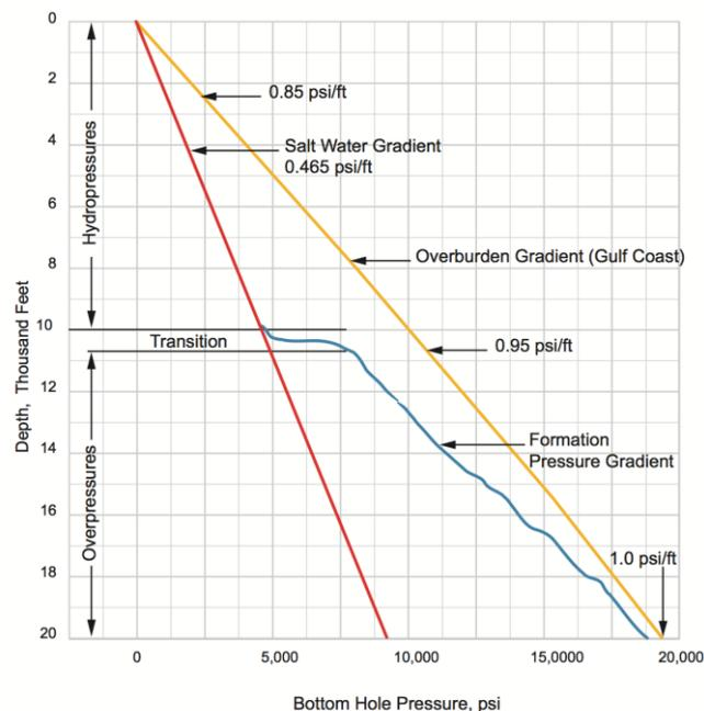
Figure 1.15 Transition from normal pressures to overpressures
