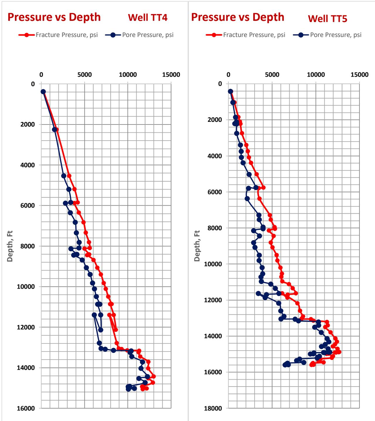
Figure 3.6 Pressure vs the depth for two wells
