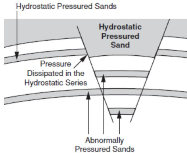
Figure 1.14 Origin of the overpressure sand and barriers to flow[24]
