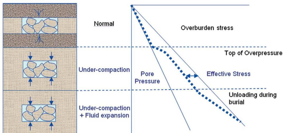
Figure 1.4 ( the formation compaction versus depth)[15]
