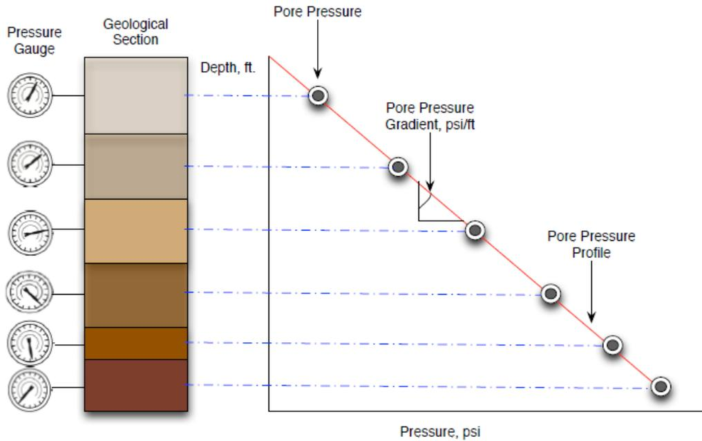
Figure 1.5 pore pressures represented in P-Z Diagram[7]
