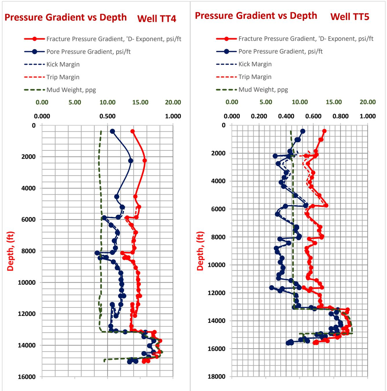
Figure 3.5 pressure gradient vs depth for two wells
