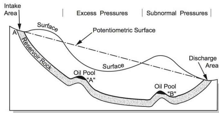
Figure 1.11 (The effect of the potentiometric surface causing abnormal pressure)[6]
