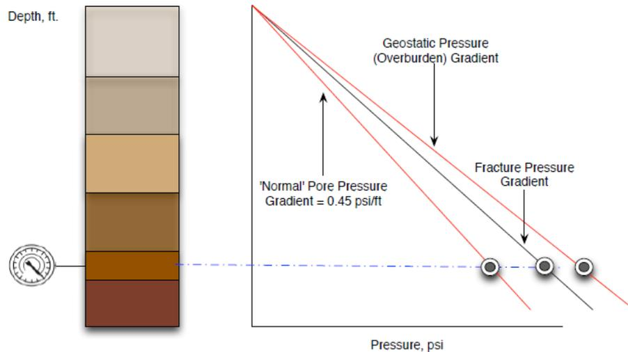
Figure 1.3 (The subsurface pressures and the gradients for each pressure ) [7]
