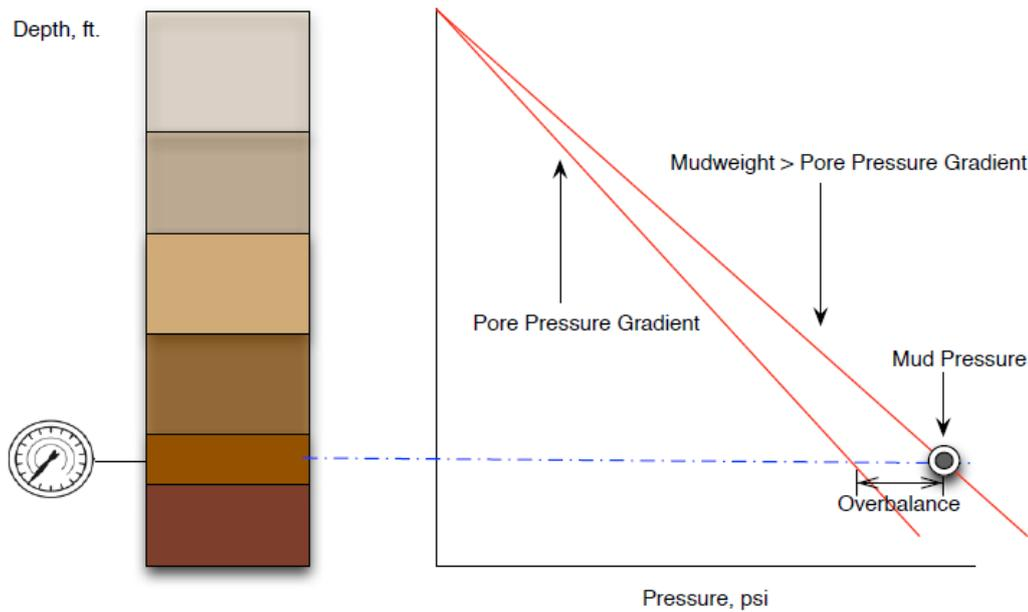
Figure 1.6 (The density of the mud versus the gradient of pore pressure)[7]
