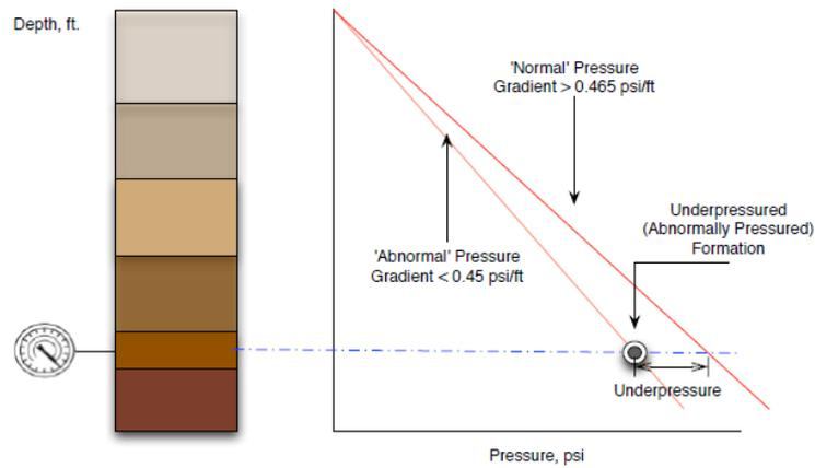
Figure 1.8 (Under pressured (Subnormal pressured) formation)[7]
