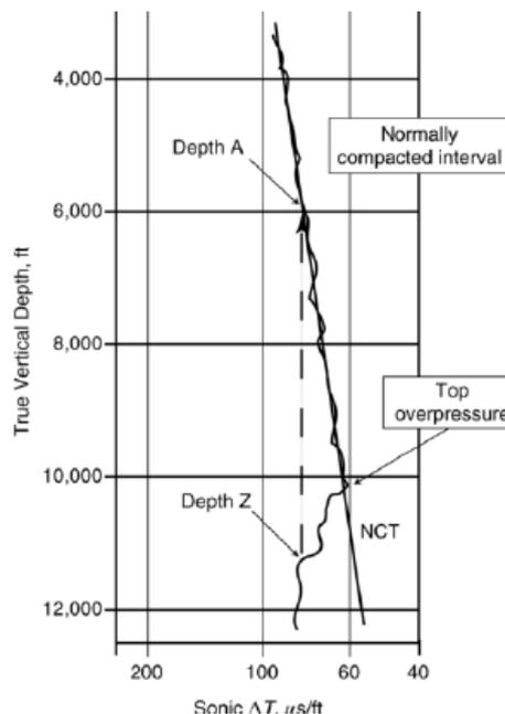
2.4 Illustration of the equivalent depth method using sonic  $\Delta T$  [37]
