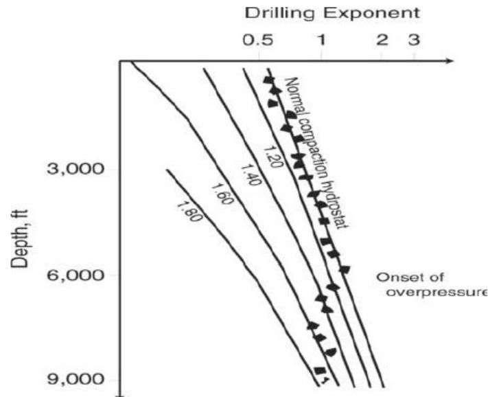
Figure 2.6 Lines for computing pore pressure using Eaton's method[7]
