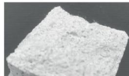
Fig. 12 Sample of the modified mortar with wool fiber incorporation
