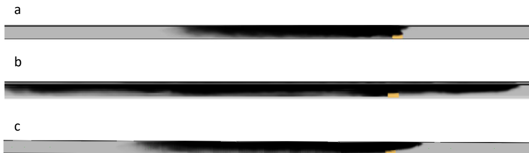
Figure 5.12: Smoke propagation with a pressure difference between portals equal to 240 Pa.
