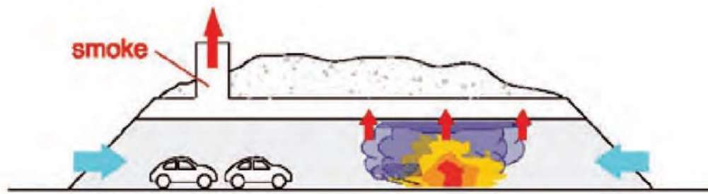
Figure 3.4: Schematic representation of semi-transverse ventilation system.
