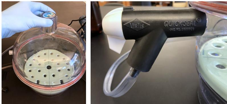
(a) Desiccator connected to the vacuum line. (b) Open valve, vacuum line is turned on.
