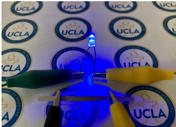
Figure 53: Emitting LED due to electrical continuity.
