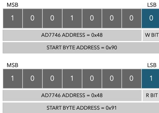
Figure 68: Start byte address for Read/Write operation.
