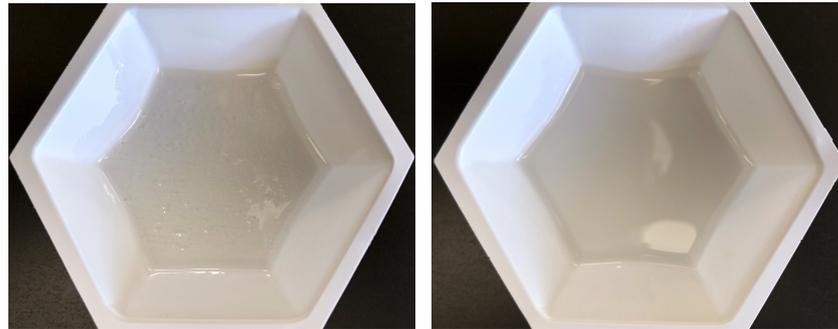
Figure 43: Produced PDMS, before and after vacuum degassing.
