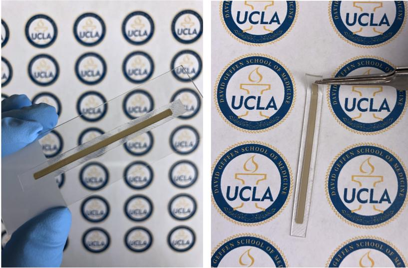
Figure 48: Conductive layer properly applied on the lower support layer.
