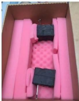
*Figure 23. Box with reference antennas. Average head mimicking liquid will be located in the middle to make it similar to the measured scenario.*
