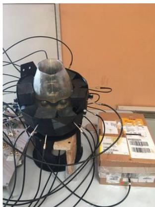
Figure 21. Head phantom filled with "brain" surrounded by brick antennas
