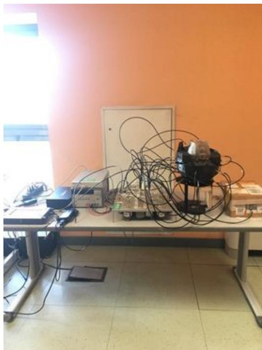
*Figure 12. Overview of MWI system at LACE. From left to right: VNA, bench power supply, switching matrix, antennas and head phantom connected through coaxial cables, box with reference antennas*
