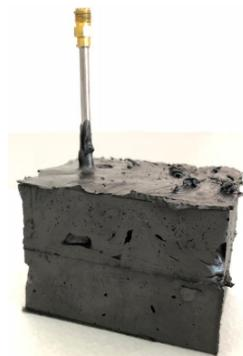
Figure 16. Brick antenna [24]
