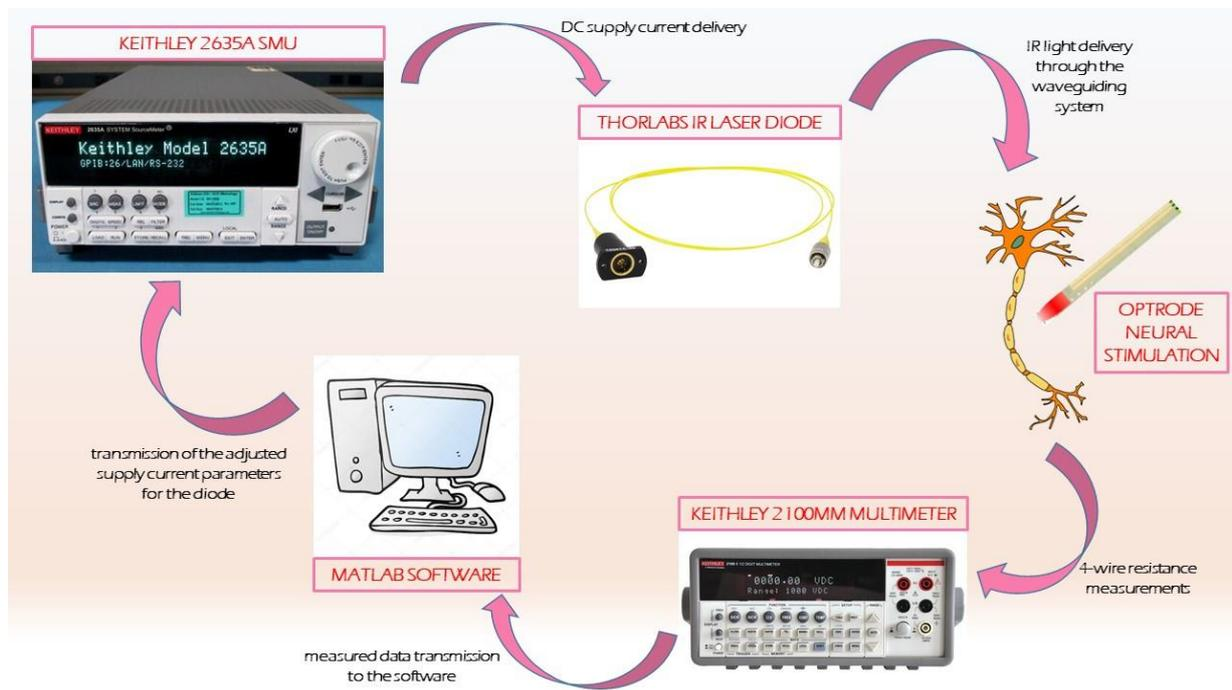
**Figure 3.3.2** The operational flow of the proposed closed-loop control in full operation.
