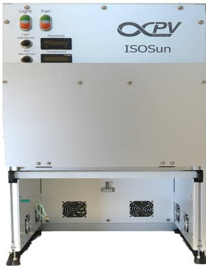
**Figure 3.9:** PV infinity ISOsun solar simulator
