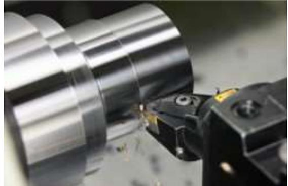
FIGURA 9 PROCESSO DI TORNITURA ESTERNA [14]
