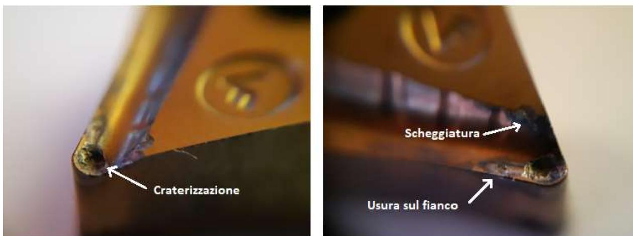
FIGURA 47 USURA DEL DNMG 150608 L-VF TT8125 A 260M/MIN
