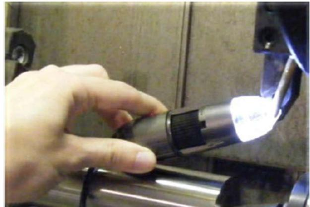
FIGURA 42 MICROSCOPIO DIGITALE HD PORTATILE (FINO 200X) [2]
