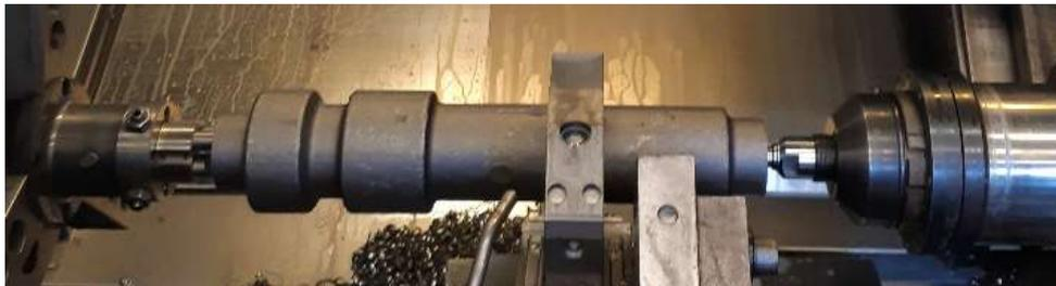
FIGURA 13 SISTEMA DI BLOCCAGGIO CON TRASCINATORE E CONTROPUNTA
