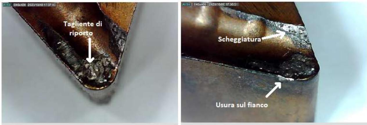
FIGURA 46 USURA DEL DNMG 150608 L-VF TT8125 A 220M/MIN
