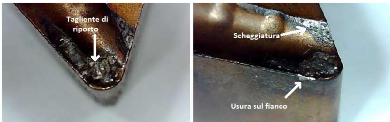
FIGURA 83 USURA A 220M/MIN: DNMG 150608 L-VF TT8125 (TAEGUTEC)
