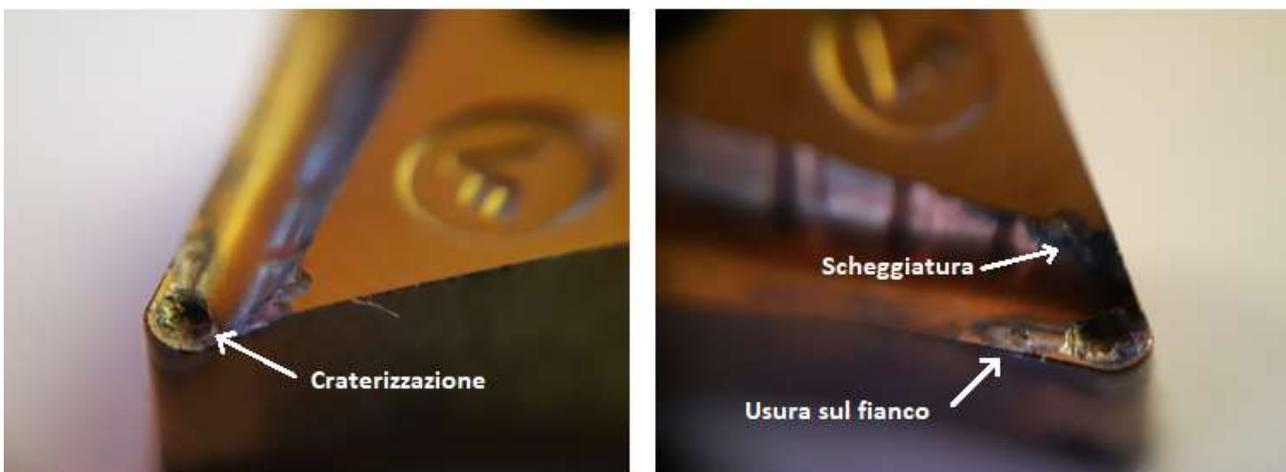
FIGURA 85 USURA A 260M/MIN: DNMG 150608 L-VF TT8125 (TAEGUTEC)
