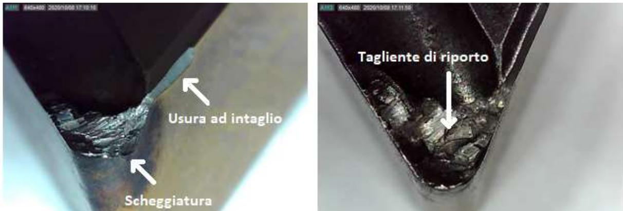
FIGURA 50 USURA DEL DNMG 150608 L-K 4415 A 220M/MIN
