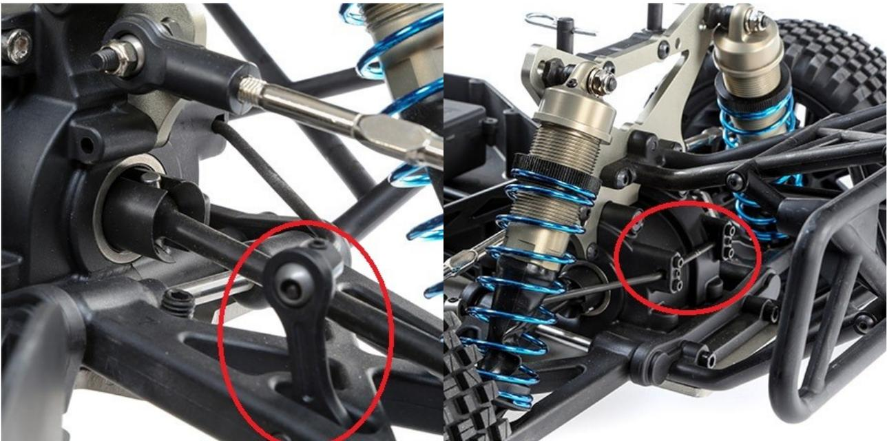
Figure 3.4.2 – Sway bar installation, hardware (left side), hooks (right side).
