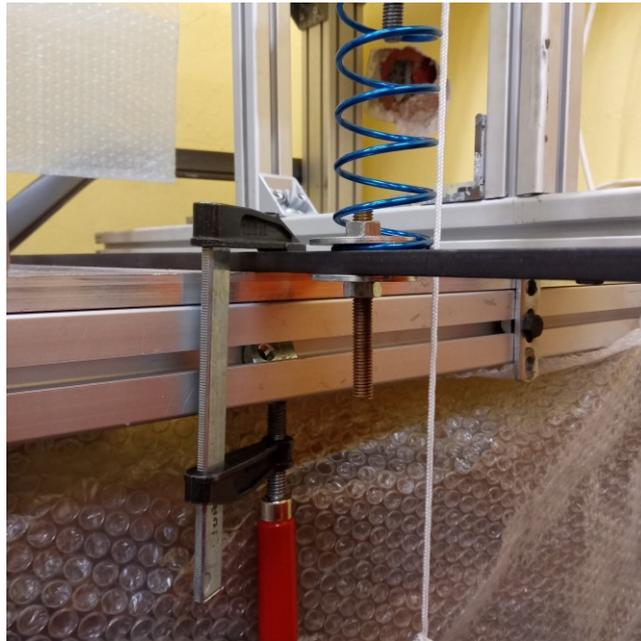
Figure 2.4.4 – Setup – clamp and low-end spring detail.
