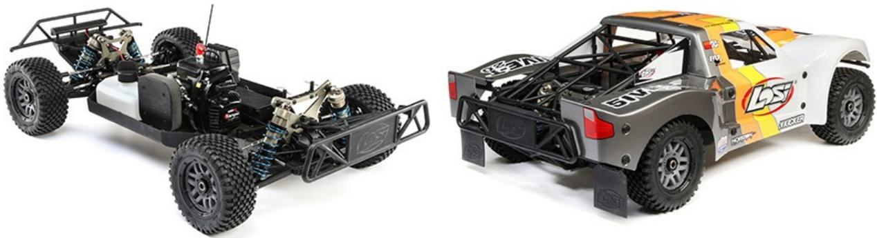
Figure 3.2 – Chassis case (left) and Body case (right).
