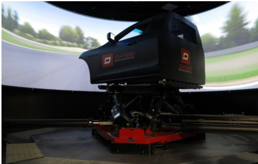
Figure 80: Danisi Engineering dynamic driving simulator [35]
