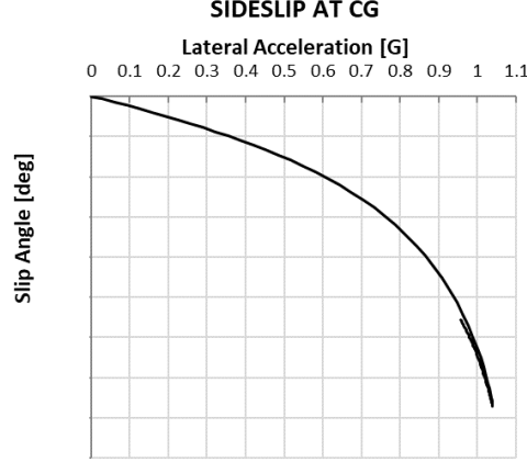
Figure 12: Side-Slip angle diagram for a ramp-steer manoeuvre
