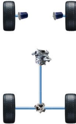
Figure 23: Hybrid vehicle powertrain configuration on VI-CarRealTime
